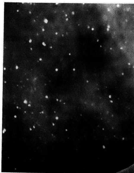
Fig. 9. BF image of the carbon layer on adsorbent A2 (magnification 20 000 ×).
