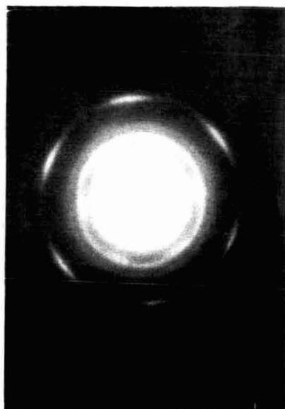
Fig. 13. DF image showing the crystalline character of the agglomerates.
