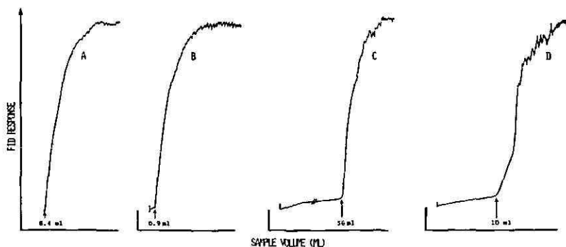
Fig. 2. Break-through curves for 0.2 ppm n -pentane in nitrogen determined at 24°C by using the flame ionization detector (attenuation, \times 32 ) to detect break-through. (A) FOTT-3, flow-rate 1 ml/min; (B) FOTT-12, flow-rate 1 ml/min; (C) FACOTT-10, flow-rate 10 ml/min; (D) FOPOTT-10, flow-rate 5 ml/min.
