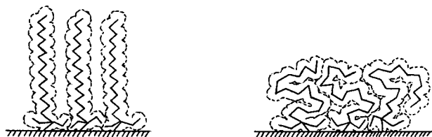
Fig. 1. “Brush” and “liquid-like” structures of bonded layer of silica modified with n -alkylsilanes.
