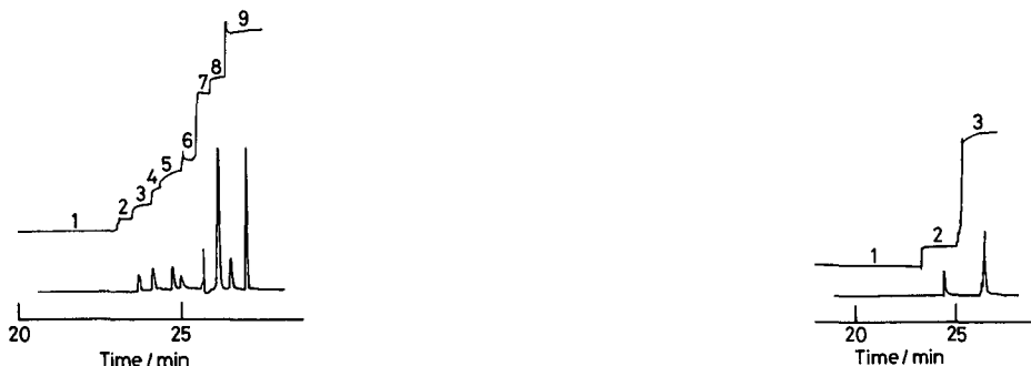
Fig. 3. Isotachopherogram of cyano-complexes: 1 = \text{Cl}^- ; 2 = copper; 3 = cobalt; 4 = silver; 5 = carbonate; 6 = zinc; 7 = cadmium; 8 = mercury; 9 = \text{CN}^- . Leading electrolyte, 5 mM hydrochloric acid-Tris, 0.005% poly(vinyl alcohol) (pH 7.5). Sample size, 10 \mu\text{l} of a mixed solution of 0.5 mM. Driving current, 50 \mu\text{A} .
