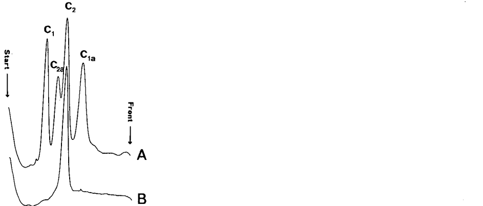
Fig. 3. HPTLC of (A) the gentamicin C complex and (B) the eluted C 2 fraction according to Kunz and Jork 35 .
