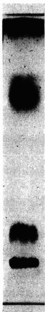
Fig. 1. Chromatogram showing the fractionation of lipid classes by TLC on sodium carbonate/Silica Gel H. The chromatogram was developed using diethyl ether–hexane–methanol (60:40:3, v/v/v) up to a height of 9 cm. The fractions are (from origin to solvent front): fatty acids (as sodium salts), monoacylglycerols, 1,2- (2,3-) plus 1,3-diacylglycerols and triacylglycerols.
