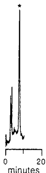
Fig. 5. Isoconfertic SFC-SCD of 28 ng of malathion (*) from a dilution in toluene of a commercial malathion formulation. Pressure at 115 atm, SFC column at 100°C. All other conditions as described in the Experimental section.
