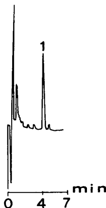
Fig. 4. Chromatogram of an urine containing 13.1 mg/l of 5-HIAA. Peak 1, 5-HIAA. Analytical conditions: column, octadecyl C_{18} 50 mm \times 4.6 mm, 3 \mu m; mobile phase 8% acetonitrile in 50 mM NaH_2PO_4 buffer pH 2.8 (8:92), containing 200 mg/l of SDS; isocratic elution; flow-rate, 1 ml/min; detector, conditioning cell, -0.20 V; det. 1, -0.20 V; det. 2, +0.25 V, gain 1 \times 2, response 2.
