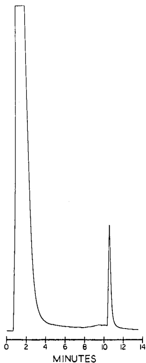
Fig. 1. Chromatogram illustrating the caffeine peak at a retention time of ca. 10.7 min.
