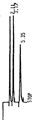
Fig. 3. Chromatogram of 0.1 mg/ml of 2 (retention time 2.11 min), ibuprofen ( 1 ) (3.17 min) and ibuproxam 3 (5.35 min) standards.
