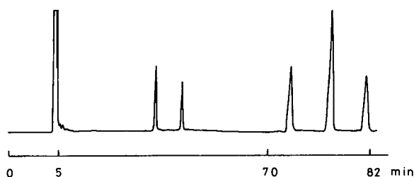
Fig. 2. GC analysis of the products of the reaction of C_6H_5POCl_2 with R,S -4-methyl-2-pentanol (after 30 min).
