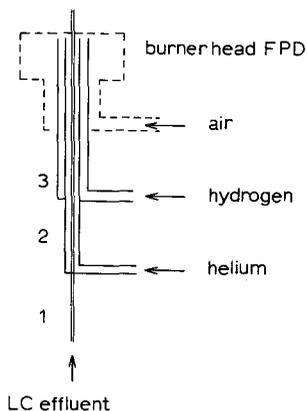
Fig. 1. Schematic interface design. 1 = Fused-silica capillary (0.10 mm I.D.); 2 = fused-silica capillary (0.32 mm I.D.); 3 = stainless-steel tube (0.50 mm I.D., 1.6 mm O.D.); 4 = burner head. For further details, see text.
