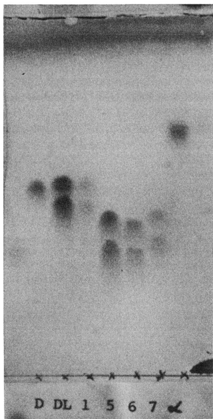
Fig. 1. Chromatogram on a Merck cellulose thin layer developed at room temperature with 0.5 M lithium chloride solution. The spots were revealed with iodine vapour. D = D-tryptophan; DL = DL-tryptophan; 1 = DL-1-methyltryptophan; 5 = DL-5-methyltryptophan; 6 = DL-6-methyltryptophan; 7 = DL-7-methyltryptophan; \alpha = DL- \alpha -methyltryptophan.
