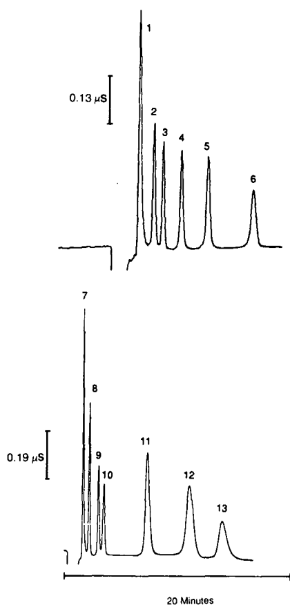
Fig. 8. Simultaneous separation of weakly and strongly acidic anions on a coupled system. Conditions: flow-rate, 1 ml/min for both separation systems; sample, 100 \mu l of a mixture of strong and weak acid anions. Other conditions were identical with those in Fig. 4 (anion exchange) and in Fig. 5 (ion exclusion). Peak identification and concentrations as in Fig. 4.
