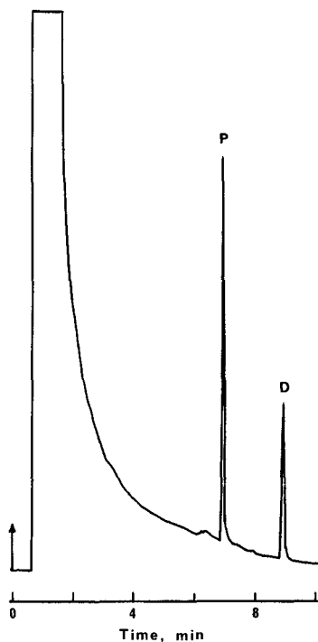
Fig. 2. Gas chromatogram of methanol extract from a commercial tablet run under conditions described in text. P = phenacetin; D = dicyclomine hydrochloride.
