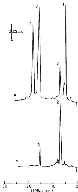
Fig. 2. HPLC of (a) 200 ng each of standard rifamycins (peaks: I = B; II = SV; III = S; IV = O) and (b) of an ethyl acetate extract from N. mediterranei fermentation broth (peaks: II = SV; III = S).
