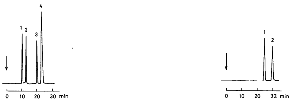
Fig. 2. Separation of a mixture of digitoxin, gitoxin, gitaloxin and internal standard I. Peaks: 1 = gitoxin; 2 = gitaloxin; 3 = digitoxin; 4 = 14\alpha,15\alpha -epoxy- \beta -anhydrodigitoxin. Conditions: Chemcosorb 5 C_8 -U column (150 mm \times 4.6 mm I.D.); mobile phase, acetonitrile-methanol-water (4:4:5); flow-rate, 0.5 ml/min; UV monitor at 220 nm; sample volume, 10 \mu l.
