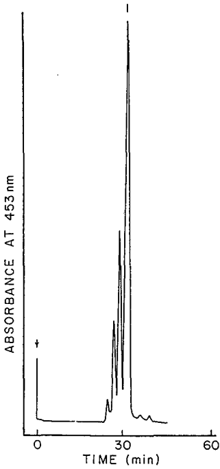
Fig. 5. SFC separation of all- trans alpha-carotene (1) and various cis isomers.
