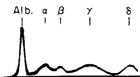
Fig. 1. Concentration distribution of blood plasma proteins following electrophoresis in a modified Tiselius moving-boundary apparatus as revealed by direct photography of the refractive index gradient by the Philpot-Svensson method. Alb. = Albumin; \alpha , \beta and \gamma = \alpha -, \beta - and \gamma -globulin; \delta is a stationary boundary.
