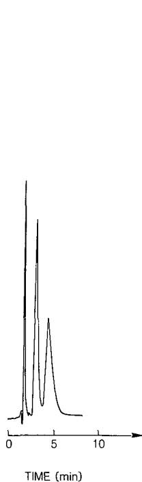
Fig. 6. Resolution of rac -benzoin on peptide column I, which contained the mixture of peptides obtained by proteolytic degradation. Column, 100 mm \times 1.6 mm I.D.; mobile phase, 0.05 M phosphate (pH 7.0); flow-rate 0.1 ml/min; UV detection at 250 nm; 0.05 \mu g injected in 0.5 \mu l of methanol. The first peak at the void volume is caused by the injected methanolic solution.
