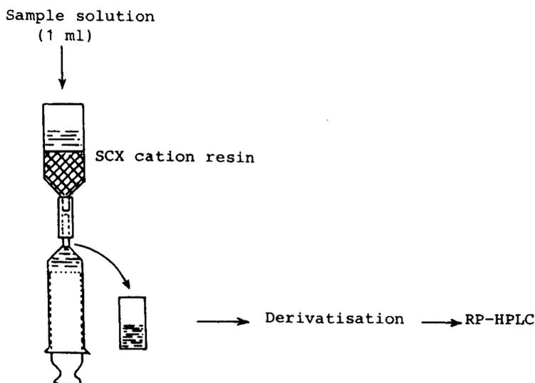
Fig. 1. Apparatus for determination of released formaldehyde.
