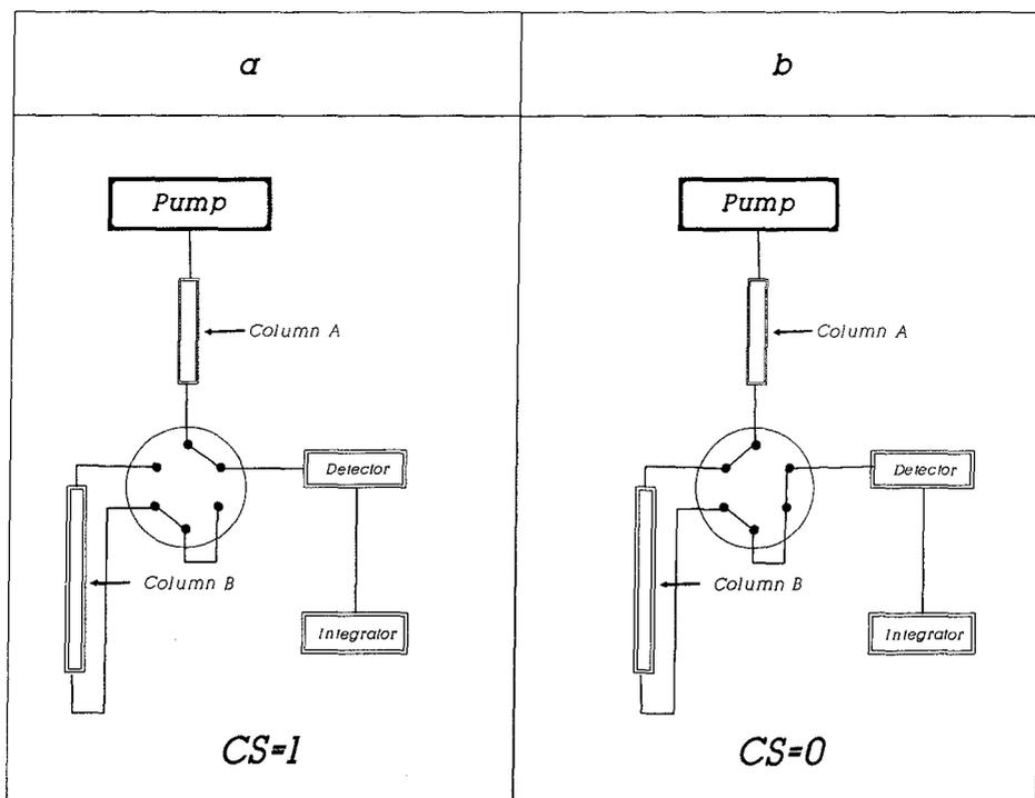
Fig. 1. Flow diagram for the determination of niacinamide. For explanations, see Experimental. (a) Separation only on column A (equal to CS = 1), (b) separation on columns A and B (equal to CS = 0).
