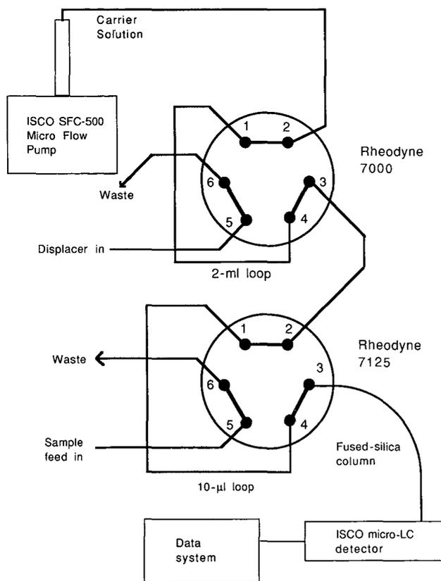
Fig. 1. Schematic diagram of the miniaturized displacement chromatographic system.
