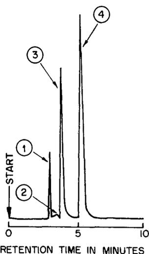
Fig. 1. Typical chromatogram of technical-grade quinalphos (30  $\mu\text{g}$ ). For conditions, see text. Peaks: 1 = *o*-xylene; 2 = epichlorohydrin; 3 = quinalphos; 4 = 1,3-dinitrobenzene (10  $\mu\text{g}$ ).
