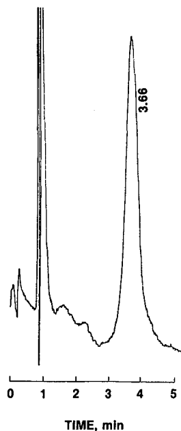
Fig. 1. Chromatogram of nitrite corresponding to 0.19 ppm in 4 ml 0.1 M sodium hydroxide eluting solution. Ambient air (180 l) was collected on a \text{C}_{18} cartridge treated with triethanolamine-sodium hydroxide and the cartridge was eluted with 4 ml eluting solution. Nitrite in the solution was determined using a Wescan Model 361 Sulfite Analyzer with an anion exclusion-HS column, a Pt working electrode set at +1.0 V vs. Ag/AgCl reference electrode. Eluent, 5 mM sulfuric acid; flow-rate, 0.8 ml/min. Injection volume, 50 \mu\text{m} . The maximum current for the nitrite peak at 3.66 min was 58 nA.
