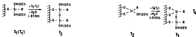
Fig. 7. Possible reaction pathways occurring after modification with octadecyltrichlorosilane. L = 2,6-lutidine (used as a catalyst); R = C_{18}H_{37} ; Et = ethyl.
