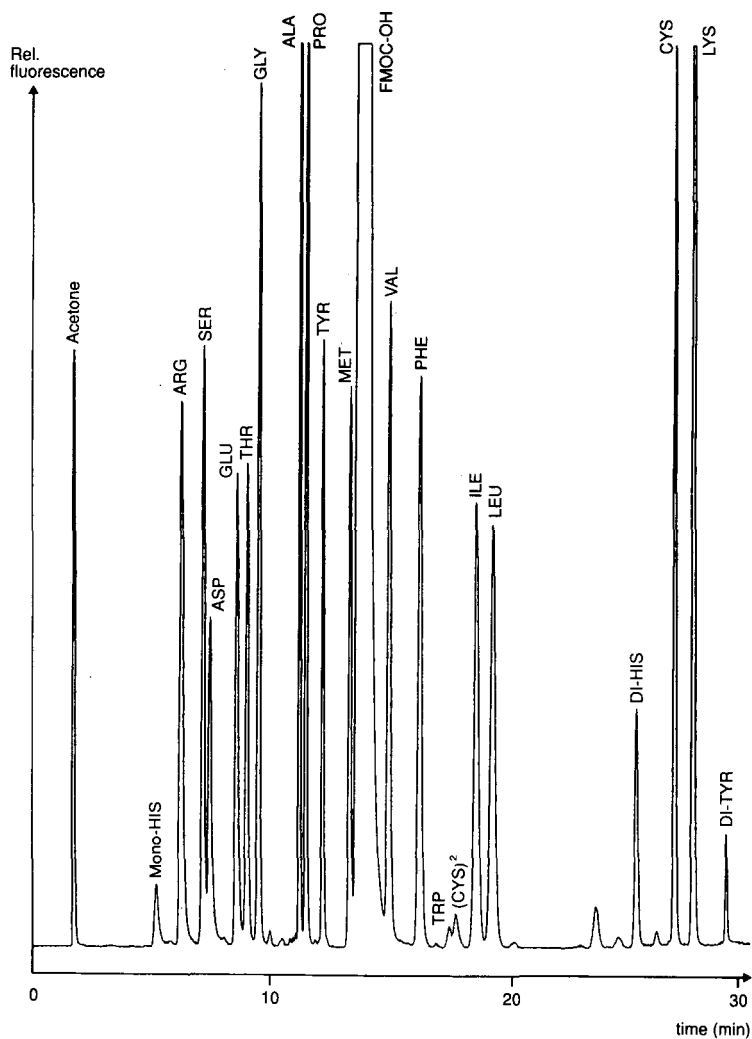
Fig. 4. Separation of protein hydrolysate standard; 10 pmol per amino acid. Fluorescence detection, \lambda_{ex} 263 nm, and \lambda_{em} 313 nm. Injection volume, 5 \mu l.
