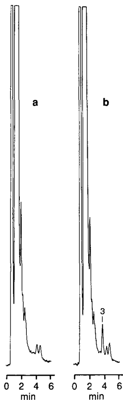
Fig. 3. Chromatograms of human plasma samples. (a) Blank plasma sample; (b) blank plasma sample spiked with 5 ng/ml of 1 . 3 is the fluorescamine derivative of 1 .
