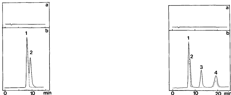
Fig. 4. Elution profiles of orthophosphate ( 1 ) and phosphonate ( 2 ). Eluent: 0.10 M KCl + 0.1% Na 4 EDTA (pH 10). Wavelength: (a) 260 nm and (b) 830 nm. The solid line in (b) indicates total phosphate and phosphonate units with sulphite and the dotted line only the phosphate unit without sulphite. Peak numbers correspond to the compound numbers in Fig. 1.
