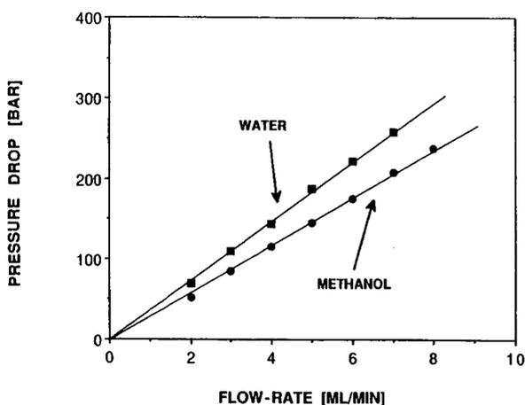
Fig. 1. Plots of pressure drop versus flow-rate of water and methanol at 25°C. Column,  $30 \times 4.6$  mm I.D. packed with  $3.3\text{-}\mu\text{m}$  micropellicular anion exchanger.
