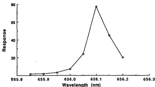
Fig. 2. Helium MIP response with  $[^2\text{H}_6]$ acetone bleed and a quartz discharge tube.
