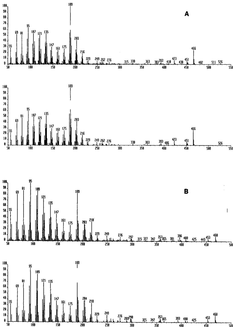
Fig. 5. Comparison of EI mass spectra of derivatives of compounds isolated from EOCl extracts (top) with those of authentic reference compounds (bottom): (A) betulin O-acetate; (B) lupeol O-acetate.
