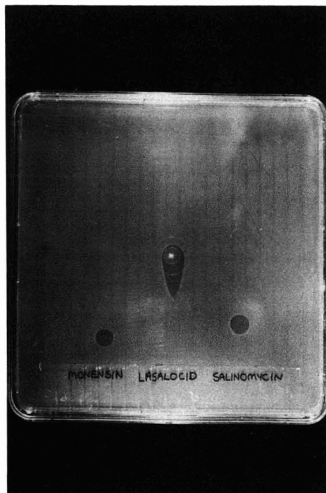
Fig. 2. Bioautogram showing TLC separation of monensin ( R_F = 0.12 ), salinomycin ( R_F = 0.21 ) and lasalocid ( R_F = 0.34 ) on pre-scored 19-channel silica gel plate.
