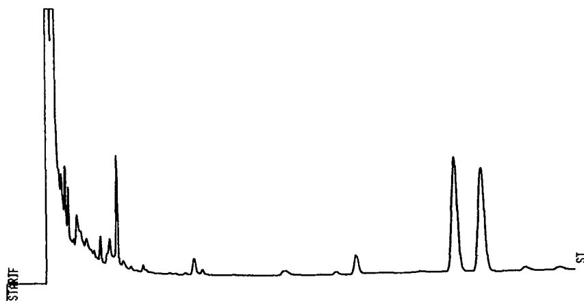
Fig. 4. Gas chromatogram of the mixed derivative in Fig. 3b. Column temperature, 250°C. Retention time for peak 2, 12 min.
