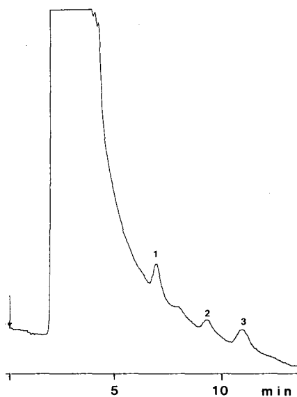
Fig. 3. Chromatogram obtained by concentrating 1000 ml of tap water spiked with 0.1 \mu\text{g/l} of dicamba (peak 1), 0.1 \mu\text{g/l} of 2,4-D (peak 2) and 0.2 \mu\text{g/l} of bentazon (peak 3) using a PRP-1 cartridge. Mobile phase: acetonitrile–water (40:60), pH 2.
