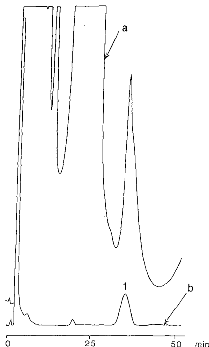
Fig. 2. Chromatograms of a fish meal sample and a standard sample using o -phthalaldehyde reagent containing thiol. (a) Fish meal (blank) (same sample as in Fig. 1a); (b) standard sample. Peak 1 = gizzerosine (10 ng), corresponding to 10 ppm in fish meal.
