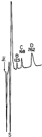
Fig. 10. Chromatogram of water extract from sample 1. The chromatographic conditions are given in Table I. Peaks: S = system peak; B = nitrate; C = chlorate; D = sulfate.
