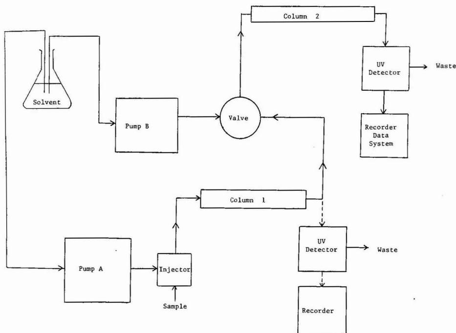
Fig. 1. A block diagram of column-switching system set-up. Pump A: 1.0 ml/min; pump B: 0.6 ml/min; column 1: RCM-100 Radial-Pak C<sub>18</sub>; column 2: Bio-Rad fast acid analysis column.
