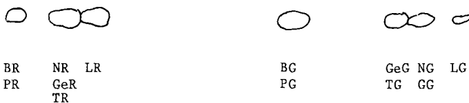
Fig. 2. OPLC of synthetic glycosidically bound volatile components on 0.2-mm silica gel (Kieselgel 60). Eluent, ethyl acetate- tert. -amyl alcohol-acetic acid-water (18:1:1:1, v/v) at a flow-rate of 0.75 ml min -1 . Nediac reagent was used for detection. Notation for glycosidically bound components as in Fig. 1.
