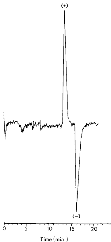
Fig. 3. HPLC separation of diphenyl-ts on (+)-poly(triphenylmethyl methacrylate)-coated silica gel. Mobile phase: methanol at a flow-rate of 0.5 ml/min; ACS ChiraMonitor.
