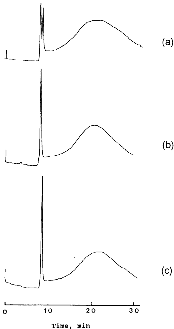
Fig. 2. Separation of diastereomeric oxazoline derivatives 2 and 3 on the \beta -CD chiral stationary phase. Mobile phase: water–methanol (9:1, v/v), pH 6.5; flow-rate: 1.0 ml/min. (a) Mixture of 2 and 3 ; (b) pure 2 ; (c) pure 3 .
