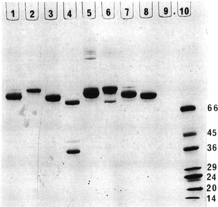
Fig. 1. Photo of 4–20% SDS-PAGE for various samples. Electrophoresis is from top to bottom. Lanes are: 1 = \alpha^- \beta^- ; 2 = \beta^- \beta^- ; 3 = \alpha^- \alpha^- ; 4 = \beta^- \beta^- plus \beta \beta ; 5 = \beta^- \beta^- ; 6 = \beta^- \beta^- ; 7 = \alpha^- \beta^- ; 8 = \alpha^- \alpha^- ; 9 = blank; 10 = protein standard mixture with indicated molecular mass (in kilodalton). The electrophoretic mobilities of the cross-linked Tm species (66 000 dalton) are lower than that of the 66 000-dalton marker on this gel system.
