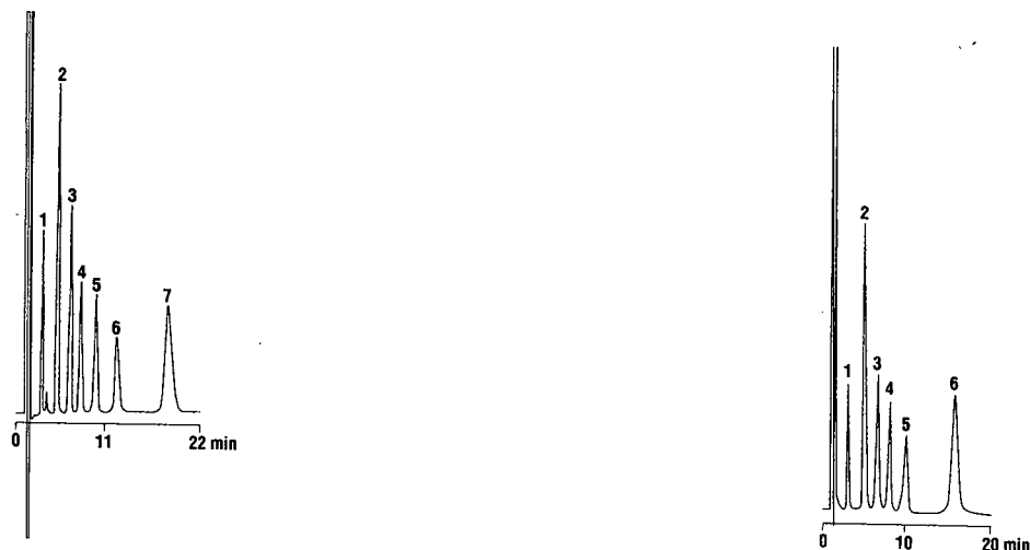
Fig. 2. Separation of the standard anion mixture using p -hydroxybenzoic acid eluent. Column, 150 mm \times 4.6 mm I.D.; packing, Alltech Universal Anion; eluent, 5 mM p -hydroxybenzoic acid, pH 7.9 adjusted with lithium hydroxide; flow-rate, 1.0 ml/min; detection, conductivity. Peaks: 1 = fluoride (10 ppm); 2 = chloride (20 ppm); 3 = nitrite (20 ppm); 4 = bromide (20 ppm); 5 = nitrate (20 ppm); 6 = phosphate (30 ppm); 7 = sulfate (30 ppm).
