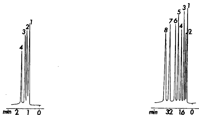
Fig. 1. Separation of C_5 hydrocarbons. Packing, -PPh_2 \cdot Ni(acac)_2 ; column temperature, 115^\circ C ; carrier gas (argon) flow-rate, 21 ml/min. Peaks: 1 = pentane; 2 = trans -2-pentene; 3 = cis -2-pentene; 4 = 1-pentyne.
