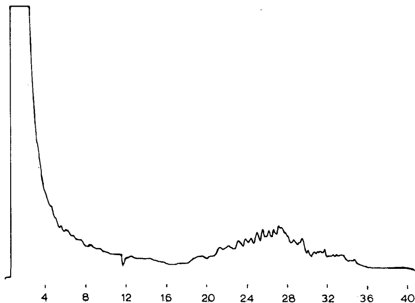
Fig. 2. On-column injection of a 100- \mu l volume without using a retention gap column. n -Pentane solution, 38°C for 17 min, then 6°C/min up to 170°C.
