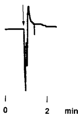
Fig. 1. Blank injection for determination of the void volume. Column: Nucleosil C_{18} (250 × 4.6 mm I.D.), 5 \mu\text{m} . Mobile phase: carbon dioxide-methanol (85:15, v/v). Temperature 22°C, pressure 15 MPa, flow-rate 3 ml/min, \lambda = 450 \text{ nm} .
