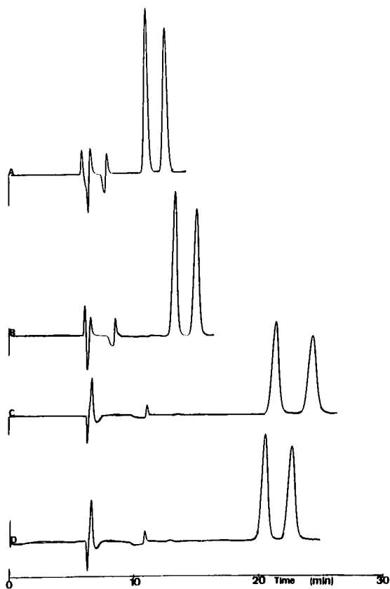
Fig. 3. Chromatograms of N-0437 (390 \mu\text{g/ml} ) obtained under various conditions: (A) eluent, hexane-ethanol (85:15), temperature 0^\circ\text{C} , flow-rate 0.5 ml/min, PO point 26; (B) eluent, hexane-ethanol (90:10), temperature 0^\circ\text{C} , flow-rate 0.5 ml/min, PO point 28; (C) eluent, hexane-ethanol (95:5), temperature 0^\circ\text{C} , flow-rate 0.5 ml/min, PO point 31; (D) eluent, hexane-ethanol (95:5), temperature 10^\circ\text{C} , flow-rate 0.5 ml/min.
