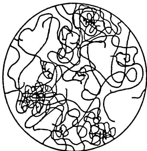
Fig. 18. Schematic presentation of the macromolecular (or matrix) structure of a lightly cross-linked polymer bead.
