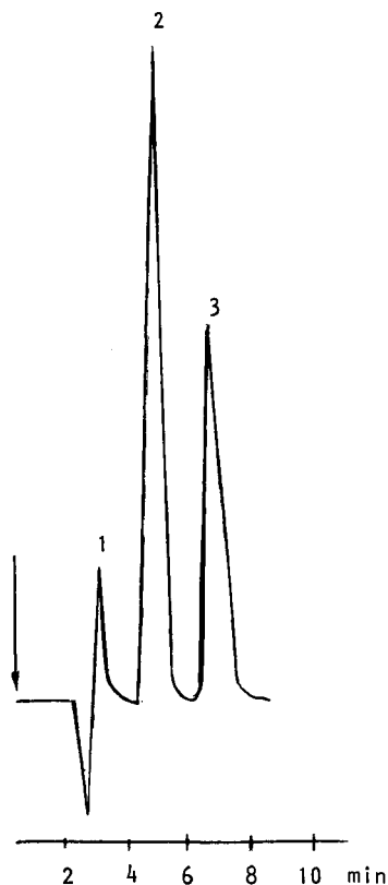
Fig. 6. Typical chromatogram of fermentation media of Corinebacterium glutamicum . Dilution, 1:50. Peaks: 1 = pyroglutamic acid; 2 = glutamic acid; 3 = glutamine. Analytical conditions as in Fig. 1.
