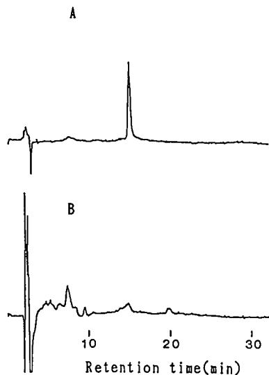
Fig. 6. High-performance liquid chromatograms. (A) Nitroxynil standard; (B) nitroxynil in raw milk sample. HPLC conditions: column, LiChrospher 100 RP-18 ( 5\ \mu\text{m} , 250 \times 4\ \text{mm} I.D.); mobile phase, acetonitrile- 0.05\ \text{M} potassium dihydrogenphosphate (20:80, v/v), pH 4.0; flow-rate, 1 ml/min at 40^\circ\text{C} . Coulometric detector: guard cell, -0.7\ \text{V} ; detector 1, -0.7\ \text{V} ; detector 2, +0.7\ \text{V} ; gain, 10 \times 40 ; response time, 10 s.
