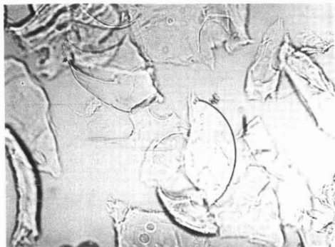
Fig. 6. Optical micrograph of ground Granocel-8 packing granules (× 90).
