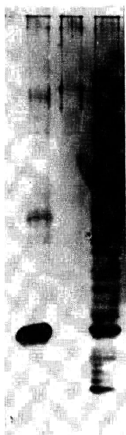
Fig. 7. SDS-PAGE of rIFN- \gamma . The large spot in the left-hand lane denotes the SDS-PAGE of the purified rIFN- \gamma from the peak at 33 min in Fig. 6. The right-hand lane represents the SDS-PAGE of the original solution extracted from E. coli cells with 7.0 mol/l GuaHCl.
