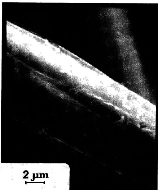
Fig. 2. Microphotograph of carbon fibres obtained from viscose, activated and impregnated with catalysts.
