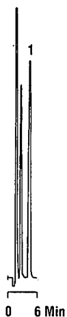
Fig. 2. Ammonia analysis of commercial emulsion explosive. Chromatographic conditions as in Fig. 1. Peak 1 = ammonium.
