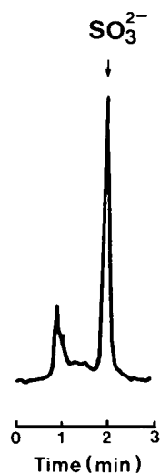
Fig. 1. Chromatogram of sulphite determined by alkali extraction–IEC method. Dehydrated apple sample. The calculated concentration in the extract is 0.56 ppm of \text{SO}_2 . Conditions: Wescan anion exclusion/HS column, eluent 20 mM \text{H}_2\text{SO}_4 ; amperometric detection (Pt, +0.6 V vs. Ag/AgCl). From ref. 31.
