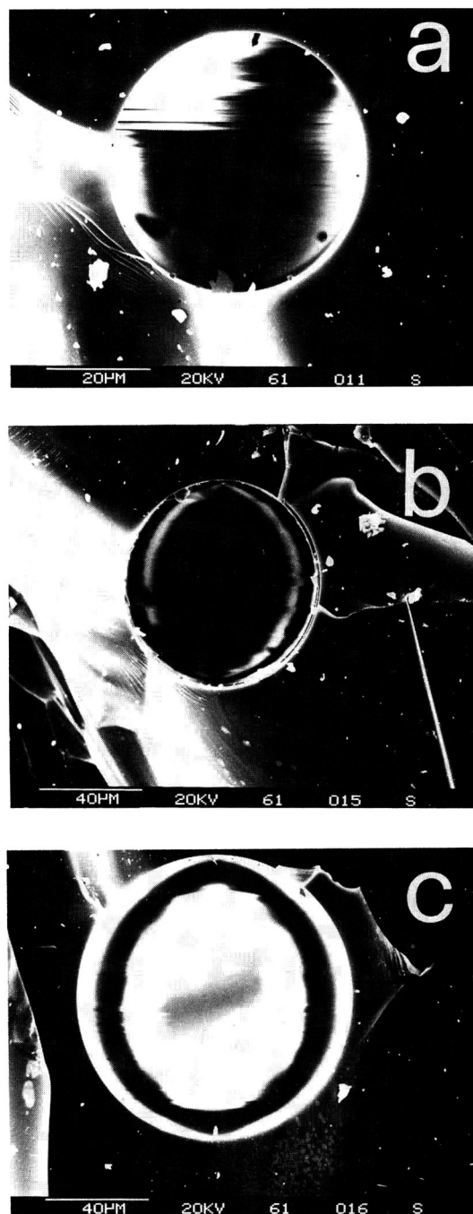
Fig. 2. Scanning electron micrographs of capillaries of different diameters: (a) 50 \mu\text{m} ; (b) 75 \mu\text{m} ; (c) 100 \mu\text{m} . Note that the round object is the lumen of the capillary. At these magnifications, only a small portion of the fused-silica wall can be seen around the lumen. The white, star-like objects are minute chips of fused-silica as a result of cutting a sharp edge.
