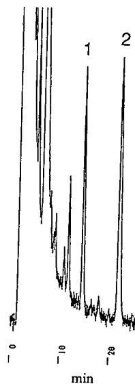
Fig. 3. HPLC separation of rac -naproxen labelled with (+)-NBD-APy. Racemic naproxen ( 1 \mu\text{M} each) and (+)-NBD-APy ( 1 \text{mM} ) in acetonitrile reacted at room temperature in the presence of DPDS ( 1 \text{mM} ) and TPP ( 1 \text{mM} ). After 2 h of reaction, the sample solution was diluted with acetonitrile and injected on to the column. HPLC conditions: column, Inertsil ODS-2 ( 150 \times 4.6 mm I.D., 5 \mu\text{m} ) at 40^\circ\text{C} ; eluent, water-acetonitrile (57:43); flow-rate, 1.0 ml/min; detection, argon ion laser at 15\text{mW} ; interference filter, 540 \pm 20 nm. Peaks: 1 = (+)-naproxen; 2 = (–)-naproxen. Each peak corresponds to 50 fmol.
