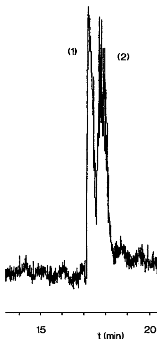
Fig. 3. CE-MS of the stereoisomers EPI (1) and DOX (2) (250 \mu\text{g/ml} each) in 10 mmol/l sodium acetate buffer (pH 7.5) and 60% methanol using a 700 \times 0.040 mm I.D. capillary and a voltage of 20 kV at the anodic end.
