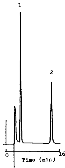
Fig. 7. Chromatogram of AA in orange juice obtained by HPLC with ED at 300 mV versus an Ag/AgCl reference electrode. Amount of AA injected, 6.33 ng in 20 \mu l. HPLC was carried out on a 15 \times 0.46 cm I.D. column of Inertsil ODS-2 (5 \mu m) using 100 mM KH 2 PO 4 (pH 3, adjusted with phosphoric acid)–1 mM EDTA·2Na as the mobile phase at a flow-rate of 0.6 ml/min at ambient conditions. Peaks: 1 = AA; 2 = I.S.
