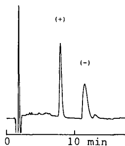
Fig. 3. HPLC separation of racemic 1-phenyl-2-( p -tolyl)ethylamine with phase I. Chromatographic conditions as in Table II.
