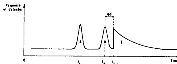
Fig. 11. Record of completely destacked sample components A and B during the separation in the L-S-L electrolyte system. In contrast to Fig. 10, where the concentration profile of the terminator shows a convex shape, the respective profile as a function of time is concave here [37]. t_{z,r} , t_{A,r} and t_{B,r} are the detection times of the front boundary of the terminating zone and of the sample zones A and B, respectively.
