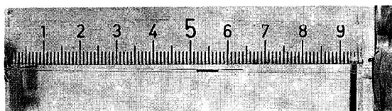
Fig. 5. Focused zone of Tessek pI Marker 6. Conditions, primary electrolyte, 0.01 M KCl; modifying electrolytes, 0.01 M KCl + 0.001 M HCl, 0.01 M KCl + 0.02 M ammonia solution; total current through column, 400 \mu A; I_H = 20 \mu A; I_{OH} = 50 \mu A. Photograph taken in 20 min.
