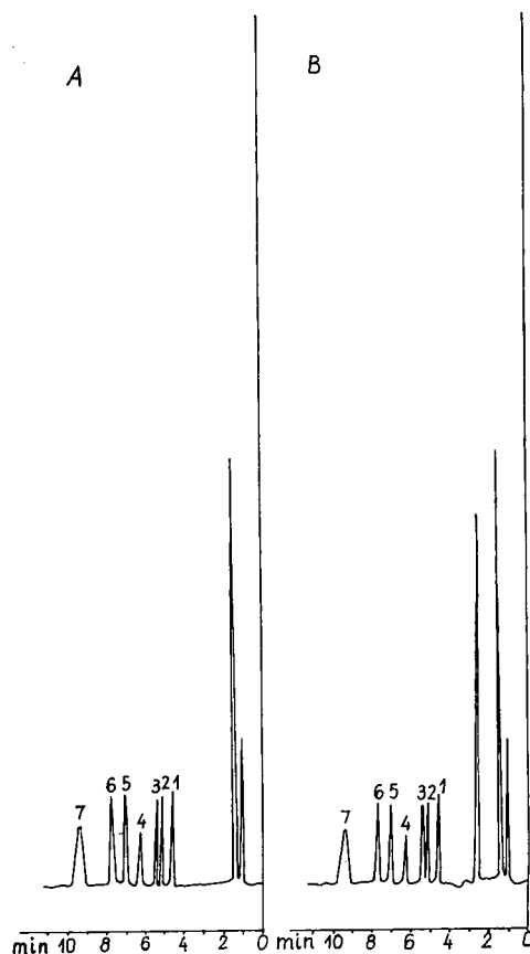
Fig. 1. HPLC chromatograms obtained by injecting (A) a mixed working standard solution of neutral and basic herbicides and (B) a tap water sample fortified with herbicides at the same concentrations. The column was a LiChrosorb-CN column and the chromatographic conditions were as described in the Experimental section. Attenuation 0.02 a.u.f.s. Peak numbering: 1 = simazine 1 ng; 2 = atrazine 1 ng; 3 = metoxuron 2 ng; 4 = monolinuron 2 ng; 5 = metobromuron 5 ng; 6 = diuron 5 ng; 7 = linuron 5 ng.
