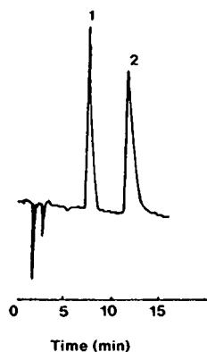
Fig. 2. Ion chromatogram of swimming pool sample treated with TCICA. Conditions: column, Omnipac PAX-100; injection volume, 10 \mu l; mobile phase, 28.8 mM sodium hydroxide-3.5% methanol; flow-rate, 1.0 \text{cm}^3/\text{min} ; detection, UV 213 nm. Peaks: 1 = \text{OCl}^-/\text{NO}_3^- ; 2 = ICA.
