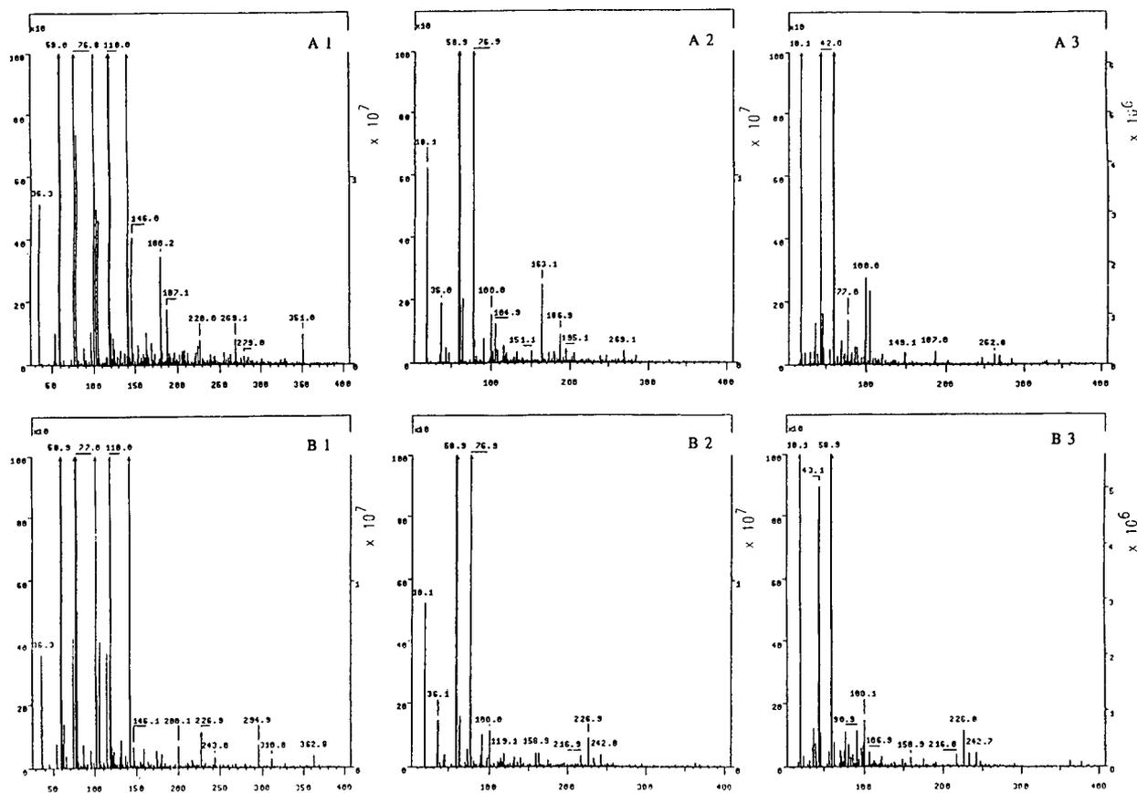
Fig. 4. Background spectra of 0.1 M ammonium acetate (or formate)-acetonitrile (ca. 90:10) in the Q3MS and RFD scan modes. (A) Acetate; (B) formate; 1 = Q3MS; 2 = RFD,  $-6$  V; 3 = RFD,  $-20$  V. Blow-up factor = 10 for all spectra.
