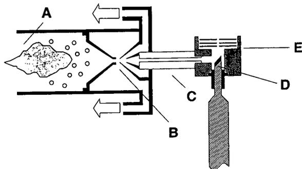
Fig. 1. Schematic representation of the LC–PB–SI–MS system. A = Desolvation chamber; B = momentum separator; C = *ca.* 15-cm transfer tube; D = surface ionization probe with platinum surface; E = ion source.
