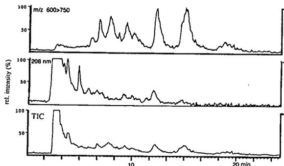
Fig. 4. LC-TSP-MS analysis of the crude dichloromethane extract of *Annona purpurea* leaves. Column, Nucleosil C<sub>18</sub>, eluent, CH<sub>3</sub>CN–H<sub>2</sub>O (85:15), at 1 ml/min; detection, UV at 208 nm; TSP: vaporizer, 90°C; source, 250°C; filament off; buffer, 0.5 M CH<sub>3</sub>COONH<sub>4</sub>, at 0.2 ml/min; 1.2 s per scan.
