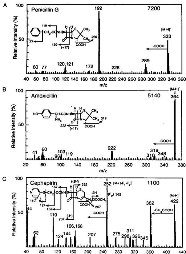
Fig. 2. Negative ion spectra of (A) penicillin G, (B) amoxicillin and (C) cephalosporin at a CAD voltage of  $-120$  V. Numbers at top right indicate ion counts.
