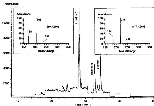
Fig. 7. On-line trace-enrichment RPLC–TSP-MS trace for river Mersey water (ions at  $m/z$  202, 216, 207 and 233 monitored). Column, 250 mm  $\times$  4.6 mm I.D. stainless-steel containing 5- $\mu$ m  $C_{18}$ -bonded silica; eluent, linear methanol–0.1 M ammonium acetate gradient [10:90 to 90:10 (v/v) in 45 min]; MS, discharge PI mode. For details, see text.
