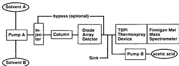
Fig. 1. Experimental set-up of the on-line RP-HPLC–diode-array UV detector–thermospray mass spectrometer system. Pump A, Waters Model 600 gradient pump; pump B, Waters M45 HPLC pump.
