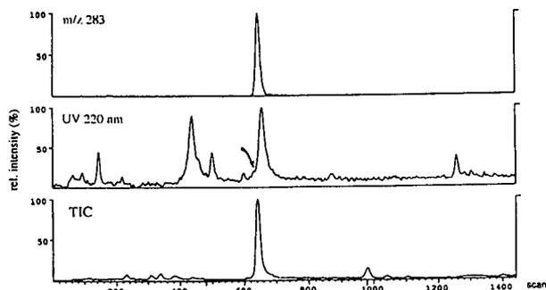
Fig. 3. LC–TSP–MS analysis of a dichloromethane extract of the aerial parts of *Artemisia annua*. Conditions as in Fig. 2. Artemisinin is indicated by an arrow in the UV trace.
