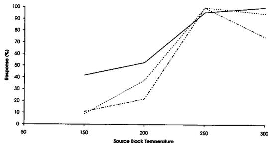
Fig. 9. Effect of source block temperature (°C) on response. Nebuliser gas pressure, 60 p.s.i.; desolvation chamber temperature, 55°C; solvent composition, methanol–water (50:50).
