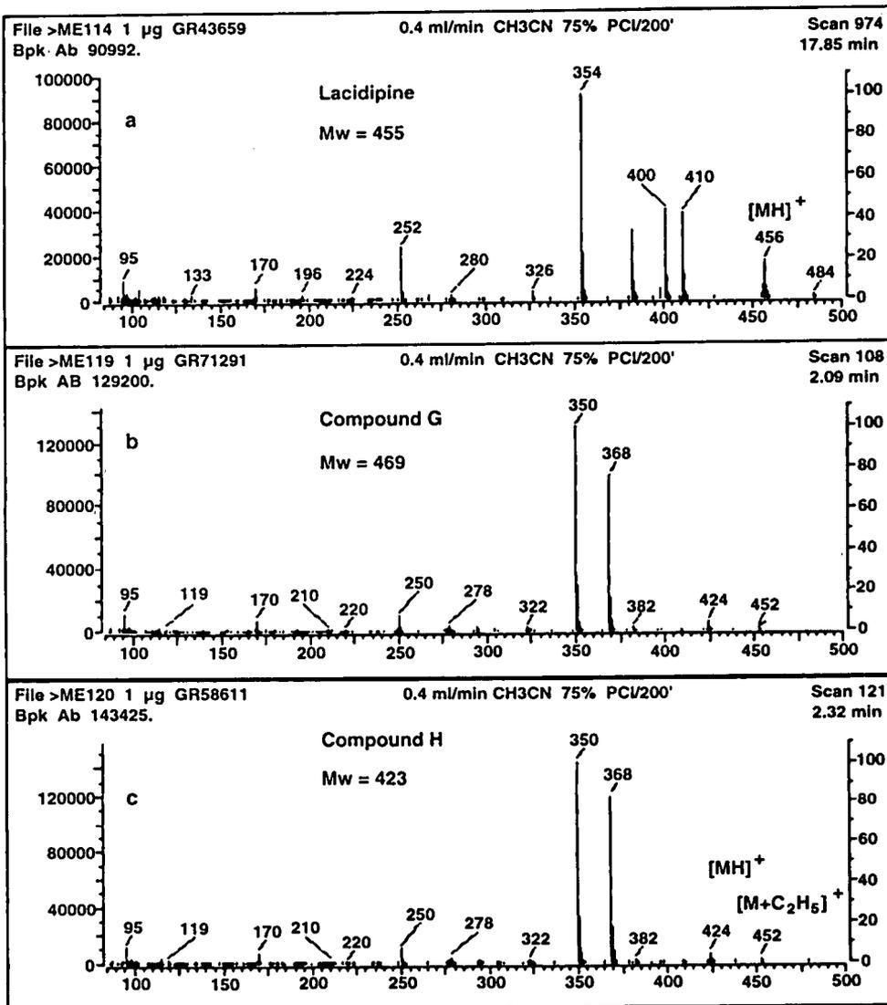
Fig. 5. PB-CI in methane, positive-ion mode, mass spectra: (a) lacidipine; (b) compound G; (c) compound H.
