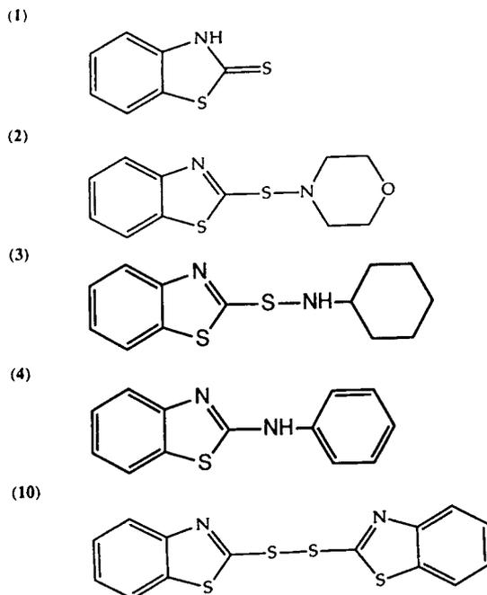
Fig. 1. Structures of the major components studied. **1** = 2(3*H*)-benzothiazolethione; **2** = 4-(2-benzothiazolythio)morpholine; **3** = *N*-cyclohexyl-2-benzothiazolesulphenamide; **4** = *N*-phenyl-2-benzothiazolamine; **10** = 2,2'-dithiobisbenzothiazole.
