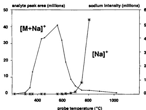
Fig. 7. Sodium background intensity and peak area for the sodiated species of several 200-ng injections of dicyclohexano-18-crown-6 ( $M_r = 372$ ) plotted as a function of the probe-tip temperature.
