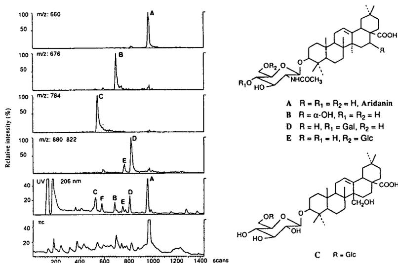
Fig. 7. LC-TSP-MS analysis of the methanolic extract from the fruits of *Tetrapleura tetraptera*. Column,  $\mu$ Bondapak  $C_{18}$ ; eluent,  $CH_3CN-H_2O$  gradient from 30:70 to 80:20 in 30 min; flow-rate 1 ml/min; detection, UV at 206 nm; TSP vaporizer, 100°C; source, 270°C; filament off; buffer, 0.5 M  $CH_3COONH_4$ , at 0.2 ml/min, 1.5 s per scan.
