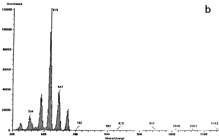
Fig. 8. LC-CI-MS spectrum of  $HRu_3(C\equiv C-C(Me)(Ph)OH)(CO)_9$ : (a) positive ion signal; (b) negative ion signal. Same conditions as in Fig. 6.
