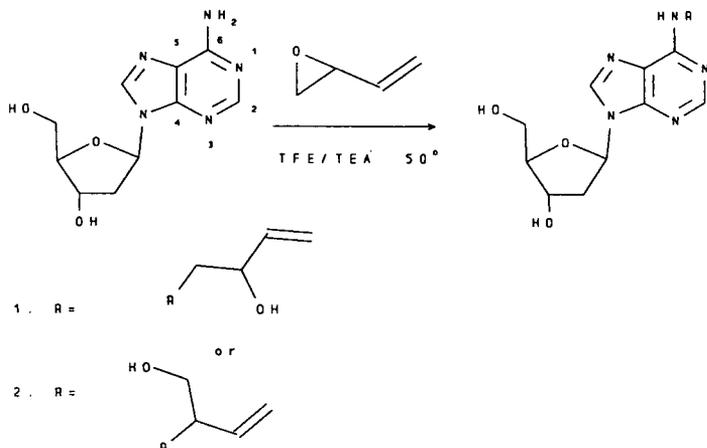
Fig. 3. Reaction of 2' deoxyadenosine and 3,4-epoxy-1-butene.
