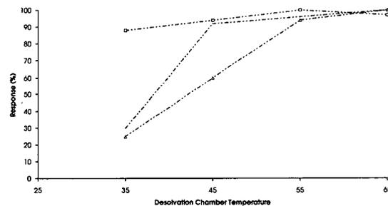
Fig. 8. Effect of desolvation chamber temperature (°C) on response (acetonitrile-water). For symbols see Fig. 1.
