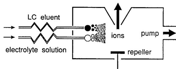
Fig. 1. Diagram of the dual-beam thermospray system.
