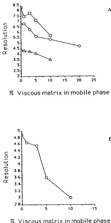
Fig. 1. Influences of FAB matrices on the resolution ( $R_s$ ) achieved in (A) conventional and (B) capillary liquid chromatographic systems. ○ = System A; □ = system B; △ = system C; ◇ = system D (see Table I).
