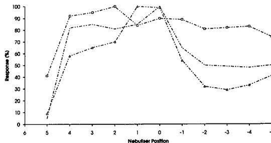
Fig. 6. Effect of nebuliser position on response at 60 p.s.i. (acetonitrile-water). For symbols see Fig. 1.
