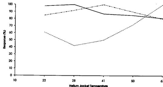
Fig. 11. Effect of heating helium on response at 60 p.s.i. Nebuliser gas pressure, 60 p.s.i.; desolvation chamber temperature, 55°C; solvent composition, methanol–water (50:50). Helium jacket temperature in °C.
