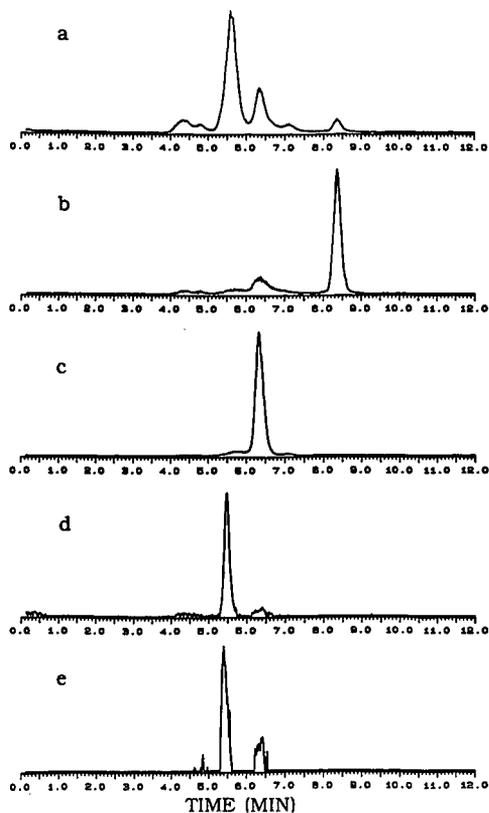
Fig. 8. Analysis of the red wine acid extract. (a) CI total ion chromatogram. Extracted ion profiles for (b) succinic acid ( $m/z$  119), (c) malic acid ( $m/z$  135), (d) tartaric acid ( $m/z$  151) and (e) citric acid ( $m/z$  193).
