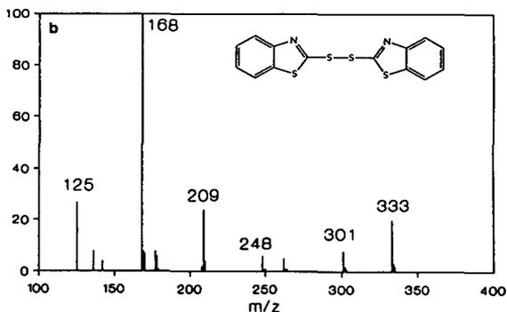
Fig. 5. Thermospray mass spectra obtained with high concentrations of (a) 2(3*H*)-benzothiazolethione (**1**) and (b) 2,2'-dithiobisbenzothiazole (**10**).
