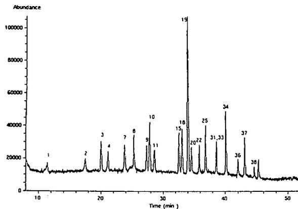
Fig. 3. RPLC-TSP-MS full-scan trace for 21 polar pesticides (150–350 u). Column, 250 mm  $\times$  4.6 mm I.D. stainless-steel containing 5- $\mu$ m C<sub>18</sub>-bonded silica; eluent, linear methanol–0.1 M ammonium acetate gradient [10:90 to 90:10 (v/v) in 45 min]; 25- $\mu$ l loop injection. For peak designation, see Table I.
