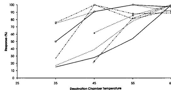
Fig. 7. Effect of desolvation chamber temperature (°C) on response (methanol-water). For symbols see Fig. 1.
