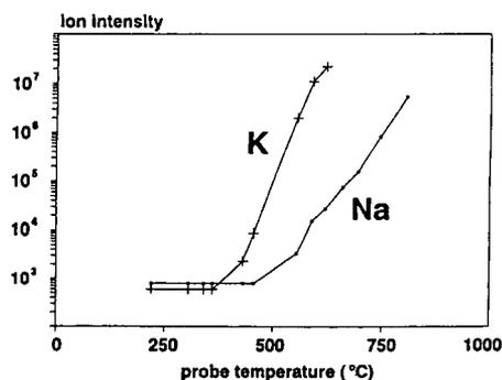
Fig. 4. Potassium and sodium background intensity as a function of the surface probe tip temperature. No liquid was introduced into the particle-beam interface.
