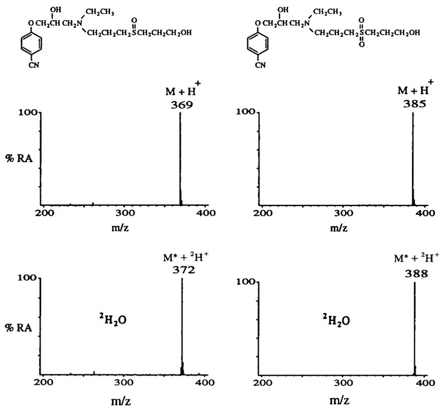
Fig. 5. Mass spectra obtained using (top) water or (bottom) deuterium oxide in the mobile phase.
