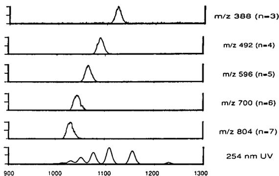
Fig. 2. GPC–MS analysis of a polystyrene A300 sample.
