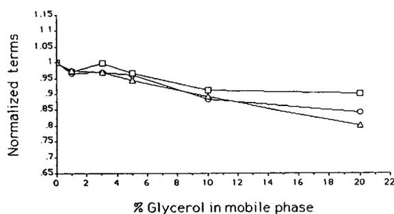
Fig. 3. Influence of glycerol on the normalized efficiency, capacity factor and selectivity terms in ion-pair chromatography (system B). ○ =  $\sqrt{N_x}/\sqrt{N_0}$ ; □ =  $f(k')_x/f(k')_0$ ; △ =  $f(\alpha)_x/f(\alpha)_0$ .
