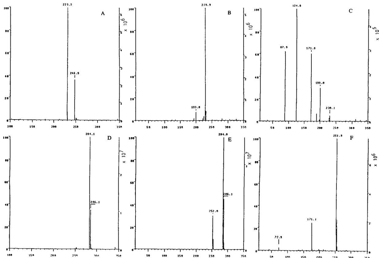
Fig. 5. Spectra of (A–C) dimethoate and (D–F) metolachlor from chromatograms in Fig. 3 after background subtraction. (A, D) Q3MS; (B, E) RFD with  $-6$  V; (C, F) RFD with  $-20$  V.
