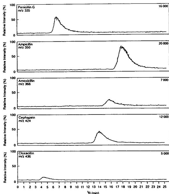
Fig. 7. Extracted ion current profiles of an microbore HPLC-ESP-MS analysis of a synthetic mixture of the five analytes at a level of 5  $\text{pg}/\mu\text{l}$  per component. Number at top right indicates ion counts of the particular mass peak seen in the ion trace. Peaks: 1 = cloxacillin; 2 = penicillin G; 3 = cephapirin; 4 = amoxicillin; 5 = ampicillin.
