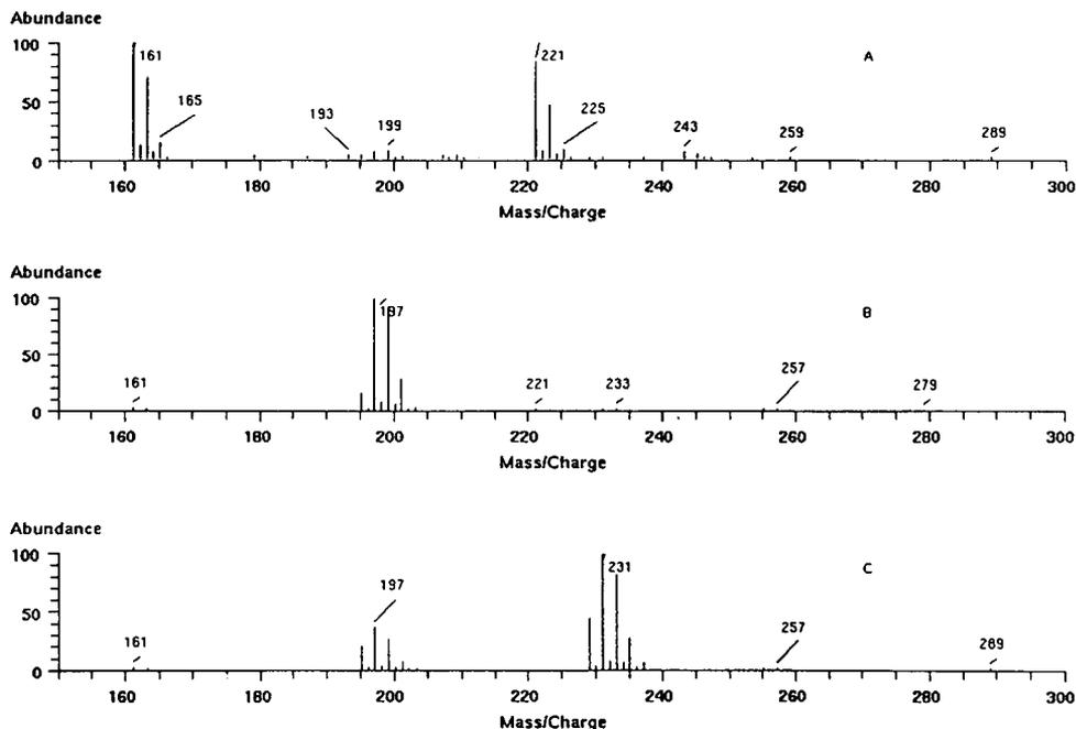
Fig. 2. TSP mass spectra of (A) 3,4-dichlorophenol, (B) 2,3,4-trichlorophenol and (C) 2,3,5,6-tetrachlorophenol in the discharge NI mode. For details, see text.
