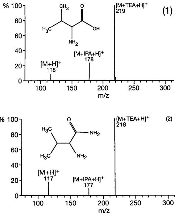
Fig. 3. Mass spectra of (1) Val and (2) Val-NH<sub>2</sub>.
