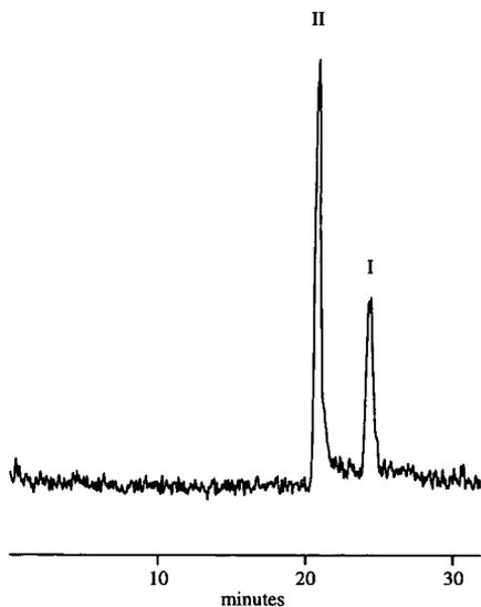
Fig. 6. Microcolumn separation of angiotensin I and II. Column, 900 mm  $\times$  0.25 mm I.D., packed with 5- $\mu$ m Kromasil C<sub>8</sub>; mobile phase, acetonitrile–5 mM ammonium acetate solution in deuterium oxide (40:60) at a flow-rate of 1.1  $\mu$ l/min. Total ion current trace obtained by scanning from 500 to 1320 u in 2 s.
