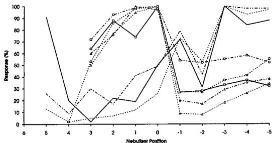
Fig. 3. Effect of nebuliser position at 40 p.s.i. (methanol-water). For symbols see Fig. 1.
