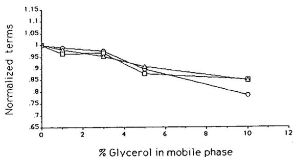
Fig. 5. Influence of glycerol on the normalized efficiency, capacity factor and selectivity terms in ion-pair chromatography (system D). ○ =  $\sqrt{N_x}/\sqrt{N_0}$ ; □ =  $f(k')_x/f(k')_0$ ; △ =  $f(\alpha)_x/f(\alpha)_0$ .
