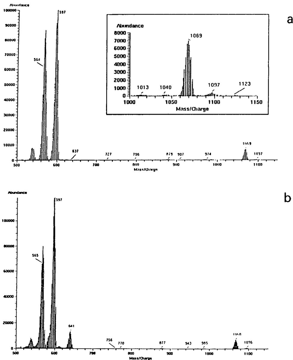
Fig. 7. Negative-ion LC–PB–MS mass spectra of: (a)  $\text{HRu}_3(\text{C}\equiv\text{C-C}(\text{Me})_2\text{H})(\text{CO})_9$ ; (b)  $\text{HRu}_3(\text{C}\equiv\text{C-C}(\text{Me})_2\text{OH})(\text{CO})_9$ . Same conditions as in Fig. 6.
