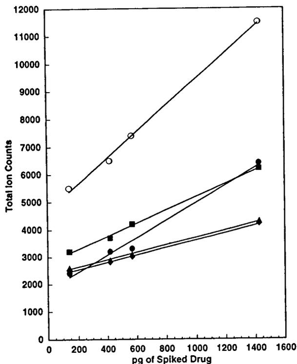
Fig. 6. Heights of peaks in total ion current profile versus amount for  $\beta$ -lactam antibiotics introduced into the mass spectrometer. ● = Penicillin G; ◆ = cloxacillin; ▲ = cephalosporin; ■ = amoxicillin; ○ = ampicillin.
