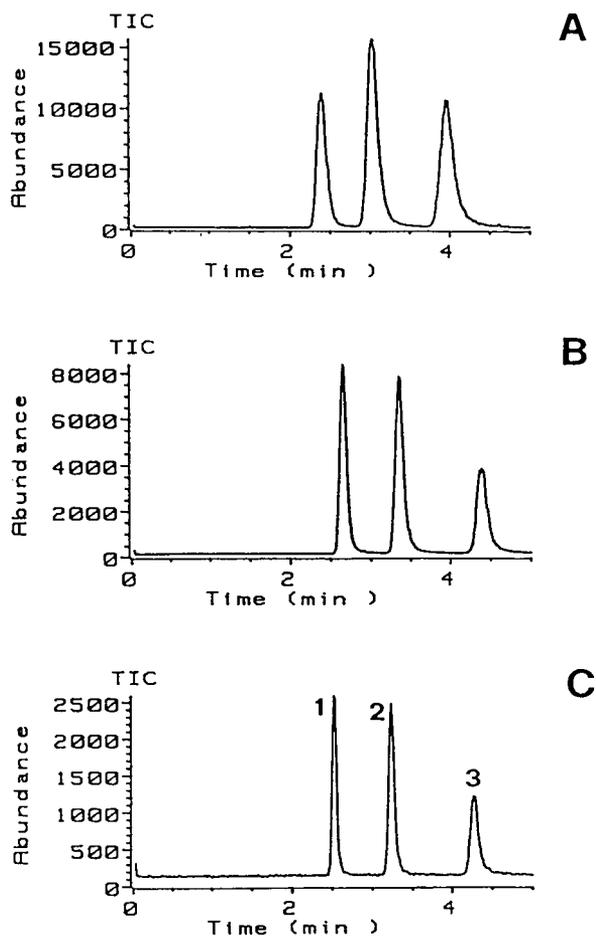
Fig. 3. LC-IS-MS traces of alkyl benzoate esters on three different column I.D.s with post-column splitting. (A) 1 mm I.D., flow-rate = 65  $\mu\text{l}/\text{min}$ ; (B) 2.0 mm I.D., flow-rate = 210  $\mu\text{l}/\text{min}$ , splitting flow-rate to mass spectrometer 65  $\mu\text{l}/\text{min}$ ; (C) 4.6 mm I.D., flow-rate = 1000  $\mu\text{l}/\text{min}$ , splitting flow-rate to mass spectrometer 65  $\mu\text{l}/\text{min}$ , injection volume 5  $\mu\text{l}$ . TIC = Total ion current.
