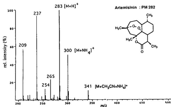
Fig. 2. TSP mass spectrum of artemisinin. Column, Nucleosil C<sub>18</sub>, eluent CH<sub>3</sub>CN–H<sub>2</sub>O gradient from 50:50 to 75:25 in 30 min; flow-rate, 1 ml/min; detection UV at 208 nm; TSP vaporizer, 90°C; source, 280°C; filament on, 600 V and 200 mA; buffer, 0.5 M at CH<sub>3</sub>COONH<sub>4</sub> 0.2 ml/min; 1.2 s per scan.
