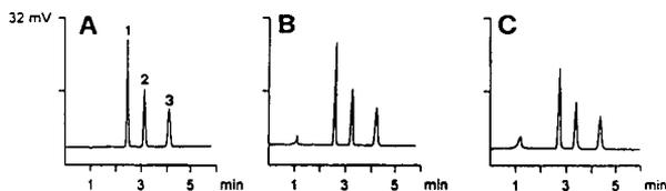
Fig. 4. LC–UV response with post-column splitting. The separation of the alkyl benzoates was performed on a  $100 \times 4.6$  mm column, UV detector with a  $2.8\text{-}\mu\text{l}$  cell, 254 nm. (A) No split, 1000  $\mu\text{l}/\text{min}$  to the detector; (B) split 5:1, 200  $\mu\text{l}/\text{min}$  to the detector; (C) split 20:1, 50  $\mu\text{l}/\text{min}$  to the detector.
