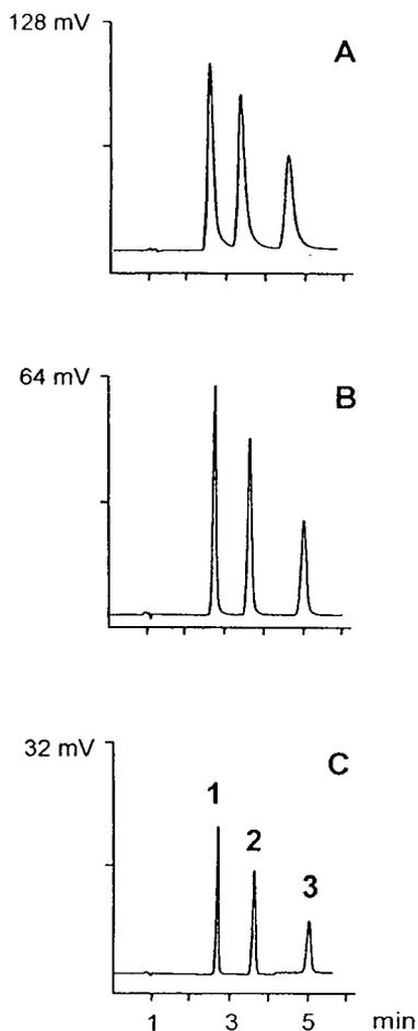
Fig. 2. LC-UV traces of alkyl benzoate esters on three different column I.D.s: (A) 1 mm I.D., flow-rate = 65  $\mu\text{l}/\text{min}$ ; (B) 2.0 mm I.D., flow-rate = 210  $\mu\text{l}/\text{min}$ ; (C) 4.6 mm I.D., flow-rate = 1000  $\mu\text{l}/\text{min}$ . UV Detector with a 0.5- $\mu\text{l}$  cell, 254 nm, 5- $\mu\text{l}$  injection. Peaks: 1 = ethyl benzoate; 2 = propyl benzoate; 3 = butyl benzoate.
