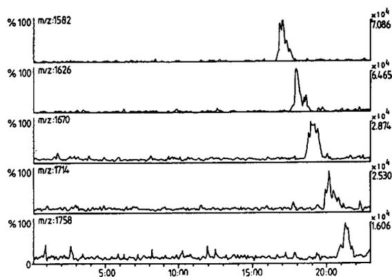
Fig. 10. Partial representation of the chromatogram for the separation of a PEG 1540 sample (200  $\mu$ g) using methanol-water 55:45 (v/v) as the mobile phase at a flow-rate of 0.5 ml/min and a 25 cm  $\times$  4.6 mm I.D. Hypersil 5- $\mu$ m  $C_{18}$  column.
