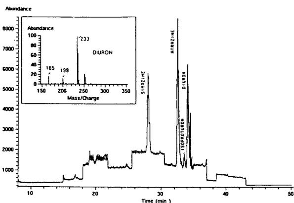
Fig. 8. On-line trace-enrichment RPLC–TSP-MS trace for river Meuse water (ions at  $m/z$  202, 216, 207 and 233 monitored). Column, 250 mm  $\times$  4.6 mm I.D. stainless-steel containing 5- $\mu$ m  $C_{18}$ -bonded silica; eluent, linear methanol–0.1 M ammonium acetate gradient [10:90 to 90:10 (v/v) in 45 min]; MS, discharge PI mode. For details, see text.
