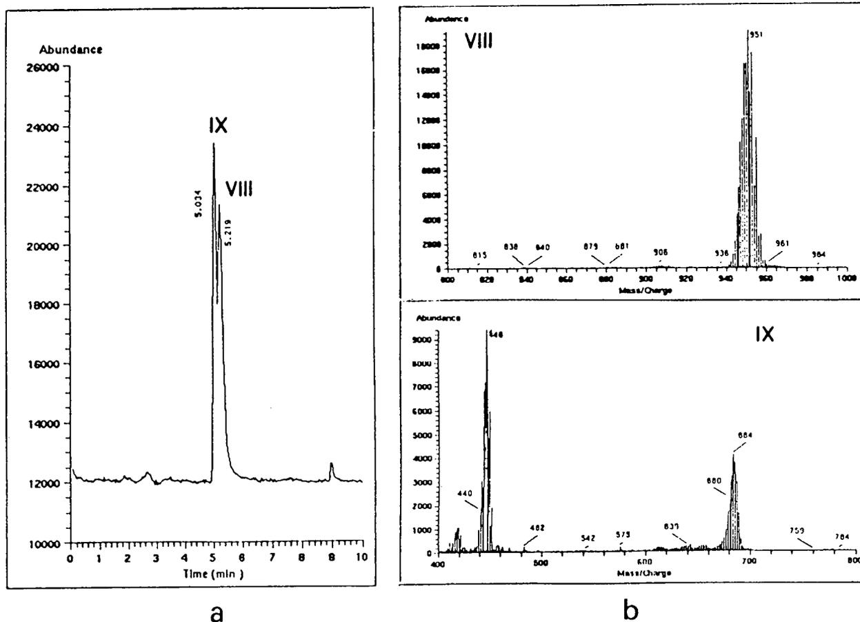
Fig. 9. (a) Separation of the nickel-ruthenium and nickel-osmium heterometallic clusters by LC-PB-MS (TIC) Chromatographic conditions: column, LiChrosorb RP-18; mobile phase, methanol; flow-rate,  $0.8 \text{ cm}^3/\text{min}$ . MS conditions as in Fig. 2, with scan range  $100\text{--}980 \mu$ . (b) MS spectra (PICI) for the clusters VIII and XI corresponding to the separation in (a).
