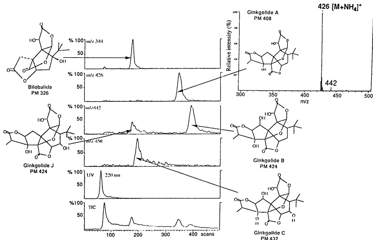
Fig. 1. LC-TSP-MS analysis of *Ginkgo biloba* extract and TSP mass spectrum of ginkgolide A. Column, Nucleosil  $C_{18}$ ; eluent, MeOH-H<sub>2</sub>O (40:60), 1 ml/min; detection: UV 220 nm. TSP: vaporizer 62°C; source 225°C; filament on, 600 V and 200 mA; buffer, 0.5 M CH<sub>3</sub>COONH<sub>4</sub> at 0.2 ml/min; 1.2 s per scan.
