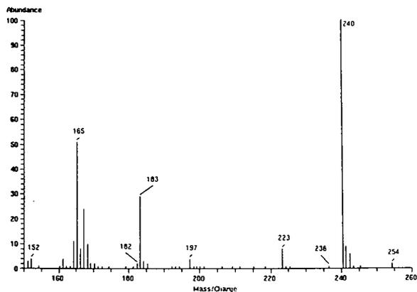
Fig. 1. TSP mass spectrum of aldicarb-sulphone in the discharge PI mode. For details, see text.
