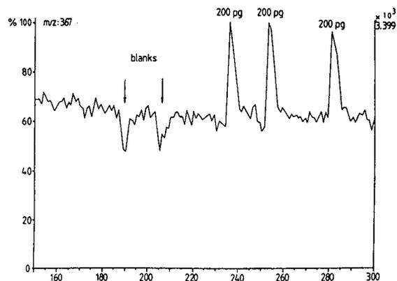
Fig. 8. Mass chromatogram for three 200-pg injections of dibenzo-18-crown-6 ( $M_r = 360$ ) with 0.5 mM lithium acetate in methanol as the mobile phase at a probe temperature of 600°C, obtained by single-ion monitoring of the  $[M + Li]^+$  intensity at  $m/z$  367.
