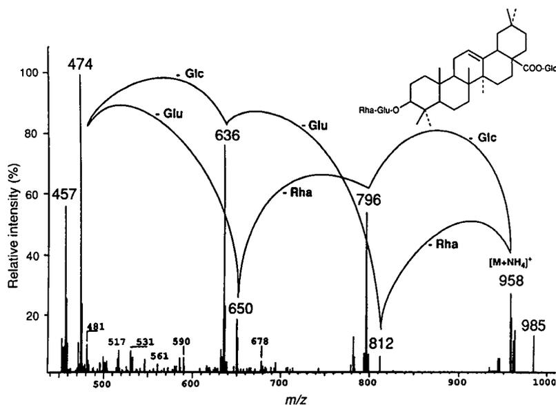
Fig. 8. TSP mass spectrum of saponin (G) obtained in the flow-injection mode. HPLC conditions: eluent,  $CH_3CN-H_2O$  (50:50); flow-rate, 1 ml/min. TSP conditions: vaporizer temperature  $100^\circ C$ ; source temperature,  $270^\circ C$ ; buffer, 0.5 M ammonium acetate; flow-rate, 0.2 ml/min; detection, UV at 206 nm.
