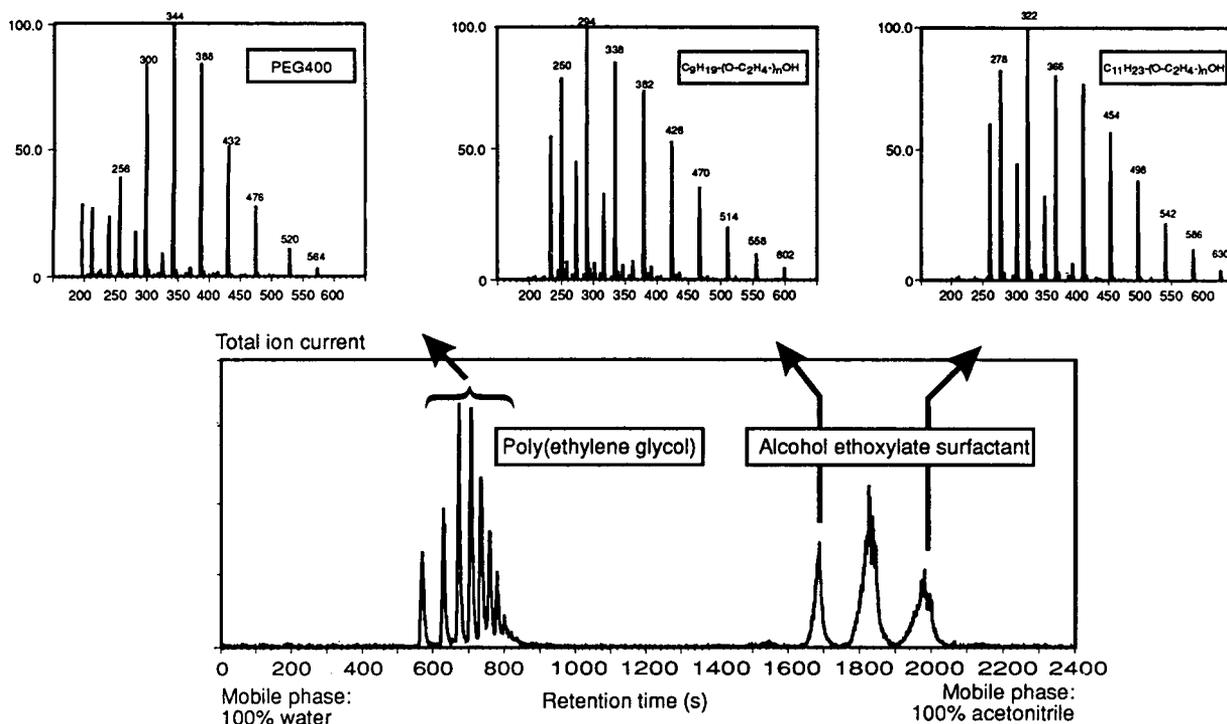
Fig. 3. Gradient elution LC-MS analysis of a mixture of polyethylene glycol (PEG400) and an alcohol ethoxylate surfactant.
