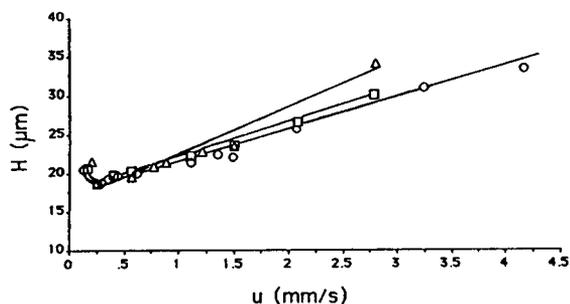
Fig. 6. Van Deemter plots for met-enkephalin at various glycerol concentrations in the mobile phase:  $\circ$  = 0%;  $\square$  = 3%;  $\triangle$  = 5%.
