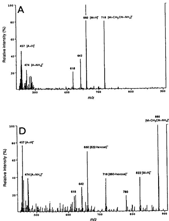
Fig. 8. TSP mass spectra of saponins A and D obtained after on-column analysis of the methanolic extract of *Tetrapleura tetraptera*. Conditions as in Fig.6.
