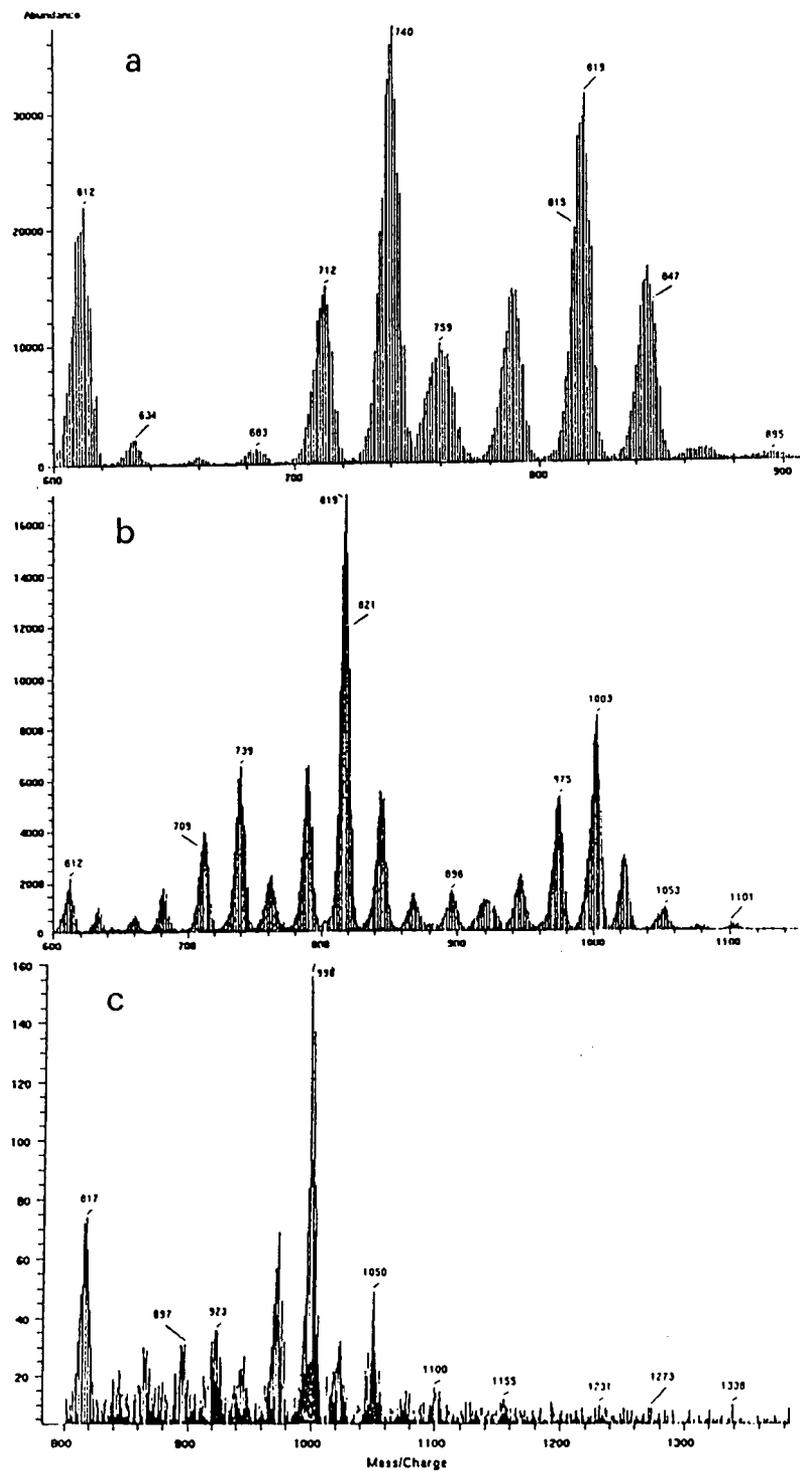
Fig. 5. LC-NICI-PB-MS mass spectra of: (a)  $\text{HRu}_3(\text{C}\equiv\text{C-tert.-Bu})(\text{CO})_8(\text{PPh}_3)_3$ ; (b)  $\text{HRu}_3(\text{C}\equiv\text{C-tert.-Bu})(\text{CO})_7(\text{PPh}_3)_2$ ; (c)  $\text{HRu}_3(\text{C}\equiv\text{C-tert.-Bu})(\text{CO})_6(\text{PPh}_3)_3$ . Conditions as in Fig. 2.
