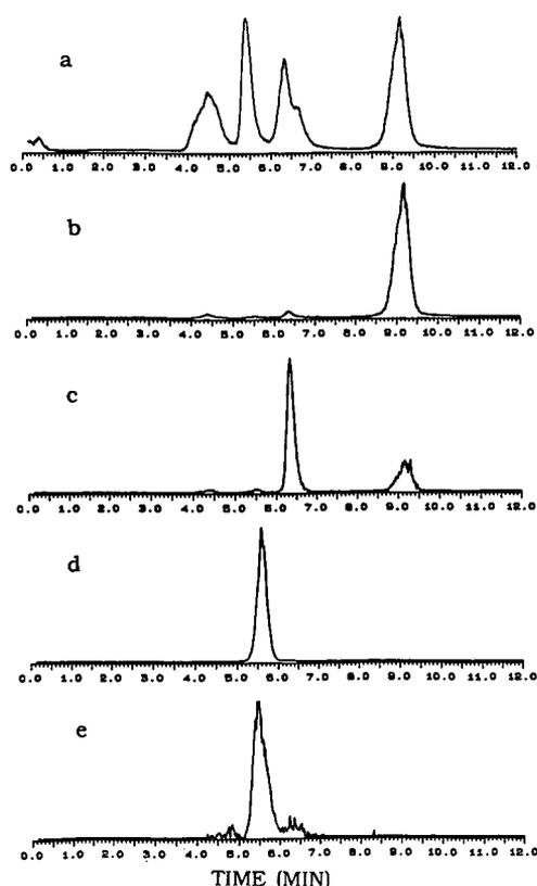
Fig. 6. Analysis of the grape juice A acid extract. (a) CI total ion chromatogram. Extracted ion profiles for (b) fumaric acid ( $m/z$  117), (c) malic acid ( $m/z$  135), (d) tartaric acid ( $m/z$  151) and (e) citric acid ( $m/z$  193).
