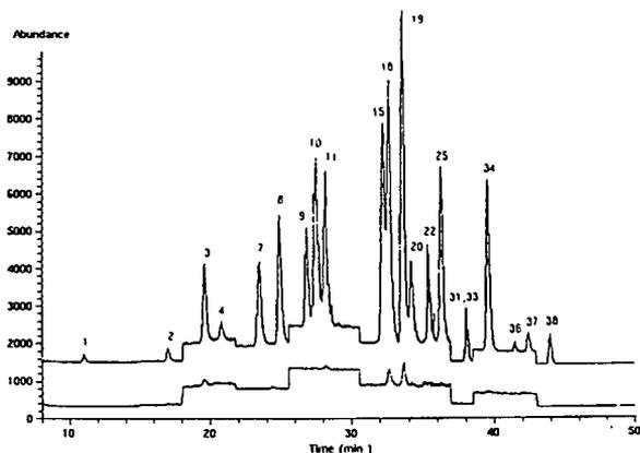
Fig. 4. On-line trace-enrichment RPLC-TSP-MS trace for 50 ml of (bottom) river Rhine water and (top) river Rhine water spiked with a mixture of 21 polar pesticides at 1  $\mu$ g/l. Column, 250 mm  $\times$  4.6 mm I.D. stainless-steel containing 5- $\mu$ m C<sub>18</sub>-bonded silica; eluent, linear methanol–0.1 M ammonium acetate gradient [10:90 to 90:10 (v/v) in 45 min]; MS, discharge PI mode. For peak designation, see Table I.
