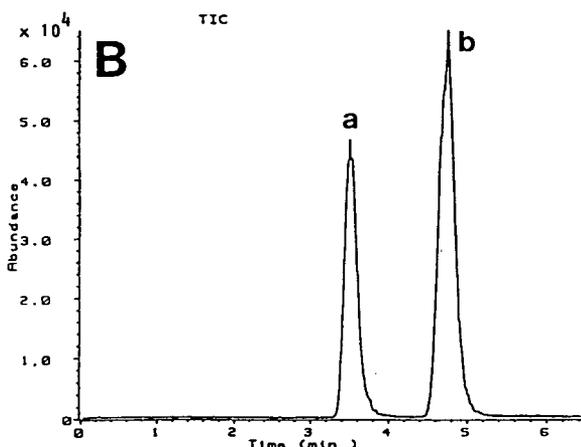
Fig. 7. SIM LC-MS response of monuron (a) and carbofuran (b) (50 ng on-column) on a  $100 \times 1$  mm I.D. column at  $50 \mu\text{l}/\text{min}$  ( $m/z = 199, 222$ , dwell time = 300 ms). (A) Conventional ion spray with no post-column addition; (B) high-flow ion spray post-column addition of  $450 \mu\text{l}/\text{min}$  using the liquid shield.
