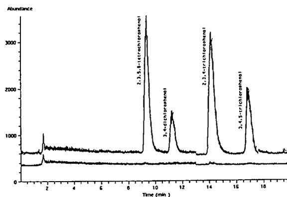
Fig. 5. On-line trace-enrichment RPLC-TSP-MS trace for 50 ml of (bottom) river Meuse water and (top) river Meuse water spiked with a mixture of four chlorophenols at 1  $\mu$ g/l. Column, 150 mm  $\times$  4.6 mm I.D. stainless-steel containing 5- $\mu$ m Rosil C<sub>18</sub>-bonded silica; eluent, linear methanol–0.1 M ammonium acetate gradient [10:90 to 90:10 (v/v) in 45 min]; MS, discharge NI mode. For details, see text.
