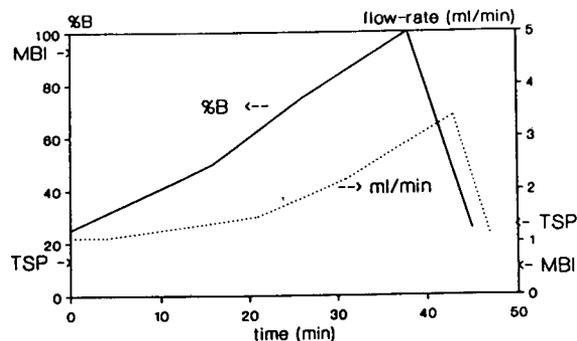
Fig. 2. Gradient elution and flow-rate programme used for the analysis of sample C. Optimum flow-rate and solvent composition conditions for the moving-belt interface (MBI) and the thermospray (TSP) interface are indicated on the abscissae.
