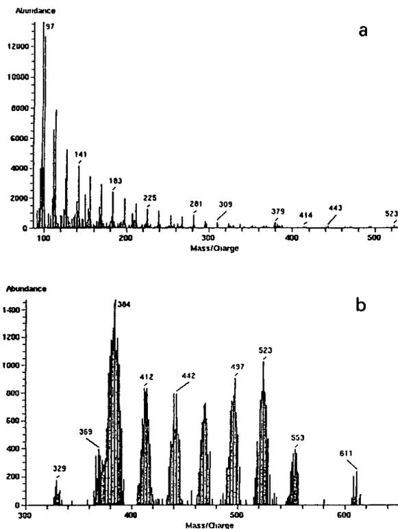
Fig. 4. LC-EI-MS mass spectra of  $\text{HRu}_3(\text{C}\equiv\text{C-tert.-Bu})(\text{CO})_9$ , at different ionization energy: (a) 70 eV; (b) 30 eV. Scan range, 150–750  $\mu$ ; electron multiplier, 2300 V; positive-ion signal.
