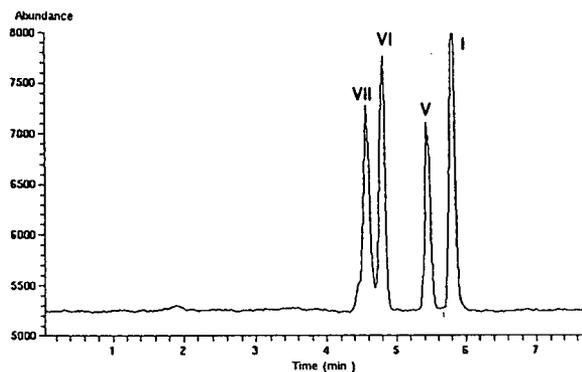
Fig. 6. Total-ion chromatogram of the cluster mixture  $\text{HRu}_3(\text{C}\equiv\text{CR})(\text{CO})_9$ . Chromatographic conditions: column, LiChrosorb RP-18; mobile phase, acetonitrile-methanol (80:20); flow-rate:  $0.8 \text{ cm}^3/\text{min}$ . MS conditions: source as in Fig. 2; NICI signal; scan range,  $150\text{--}750 \mu$ .
