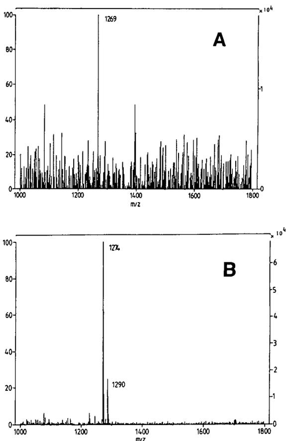
Fig. 9. Spectra from the PEG component  $HO[C_2H_4O]_{28}H$  ( $M_r = 1251$ ) of a PEG 1540 sample after chromatographic separation. (A) Obtained under CI conditions at an  $NH_3$  source pressure of 500 Pa; (B) obtained under SI conditions at a probe temperature of 1100°C at a  $O_2$  source pressure of 30 Pa.
