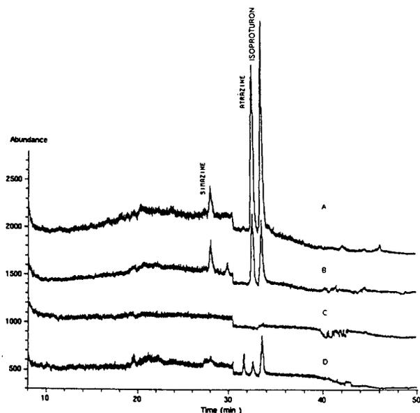
Fig. 6. On-line trace-enrichment RPLC–TSP-MS trace for 200 ml of (A) Rhine water, (B) Amsterdam drinking water, (C) blank without pre-concentration and (D) HPLC-grade water. Column, 250 mm  $\times$  4.6 mm I.D. stainless-steel containing 5- $\mu$ m  $C_{18}$ -bonded silica; eluent, linear methanol–0.1 M ammonium acetate gradient [10:90 to 90:10 (v/v) in 45 min]; MS, discharge PI mode. For details of time-scheduled SIM, see text.
