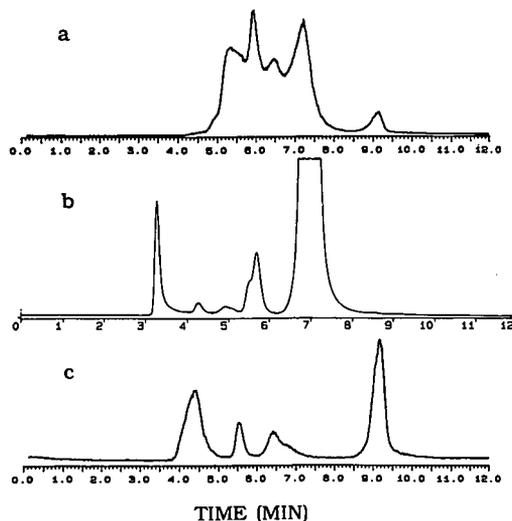
Fig. 5. Analysis of grape juice A before SAX extraction: (a) CI total ion chromatogram; (b) UV chromatogram. Analysis of grape juice A after SAX extraction: (c) CI total ion chromatogram.
