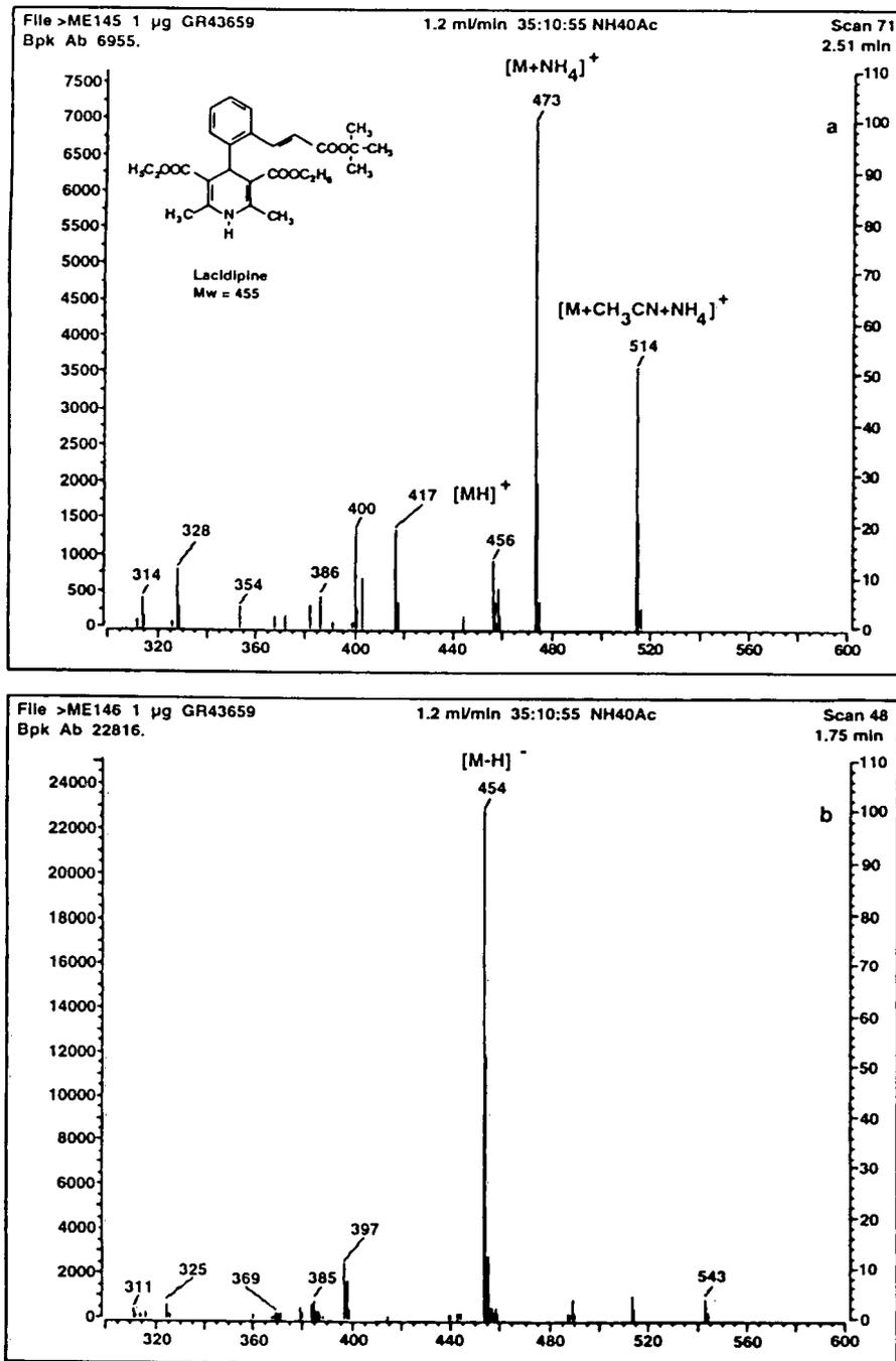
Fig. 2. Thermospray mass spectra of lacidipine: (a) positive-ion mode; (b) negative-ion mode.
