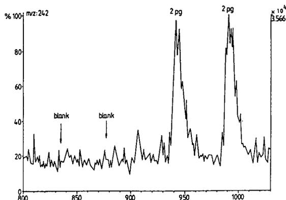
Fig. 3. TSI mass chromatogram for two injections of 2 pg of tetrabutylammonium (formula mass = 242) bromide recorded in the single-ion detection mode at  $m/z$  242, applying a probe temperature of 600°C.
