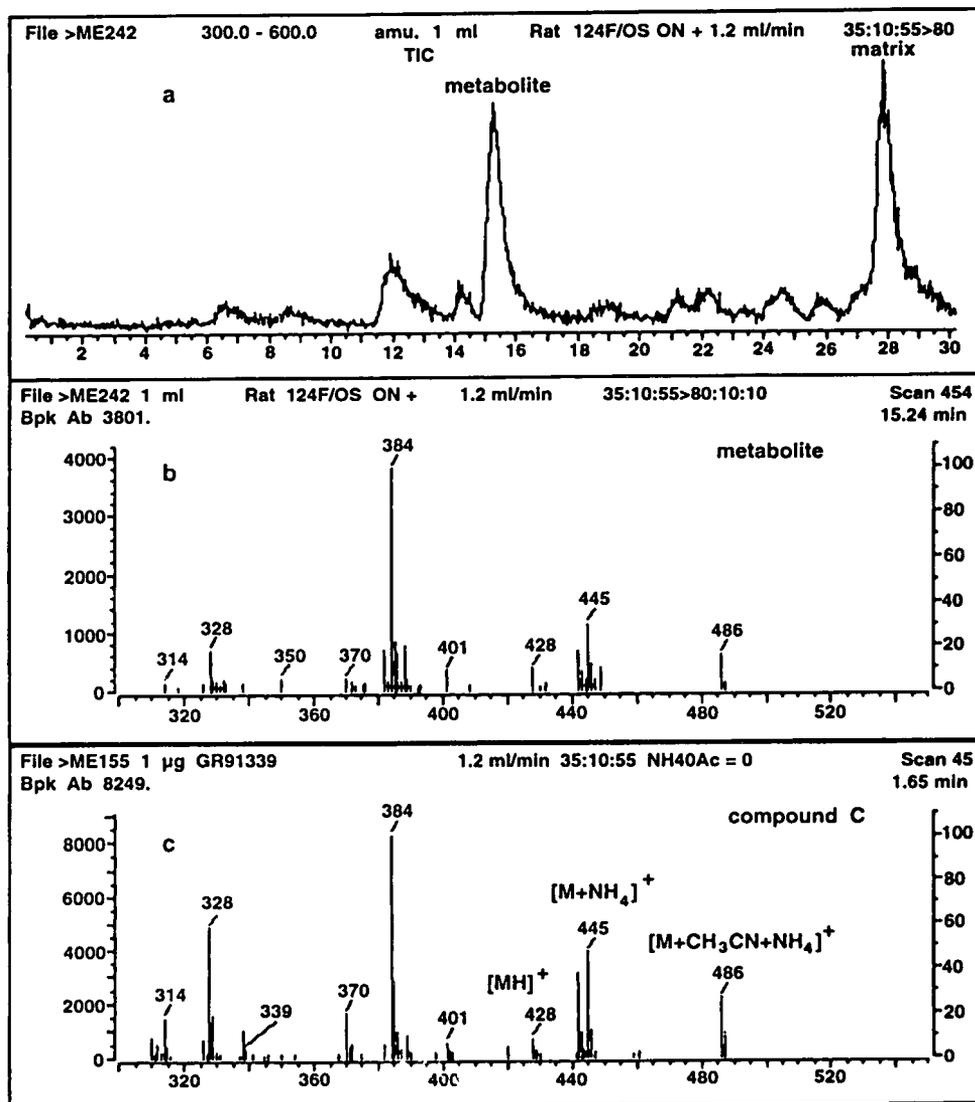
Fig. 8. HPLC-TSP-MS measurements of a rat plasma sample. (a) Total ion current (TIC) chromatogram. (b) Mass spectrum of the peak eluting at 15.2 min. (c) Mass spectrum of compound C standard.
