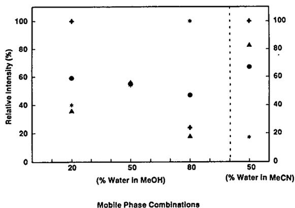
Fig. 1. Electrospray intensity for penicillin G (★) amoxicillin (+) and cephalosporin (▲) in different mobile phase combinations at a capillary-skimmer potential of +160 V. ● = Average response.
