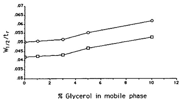
Fig. 4. Effect of concentration of glycerol in the mobile phase on the normalized peak width ( $w_{1/2}/t_r$ ).  $\circ$  = Met-enkephalin;  $\square$  = leu-enkephalin.
