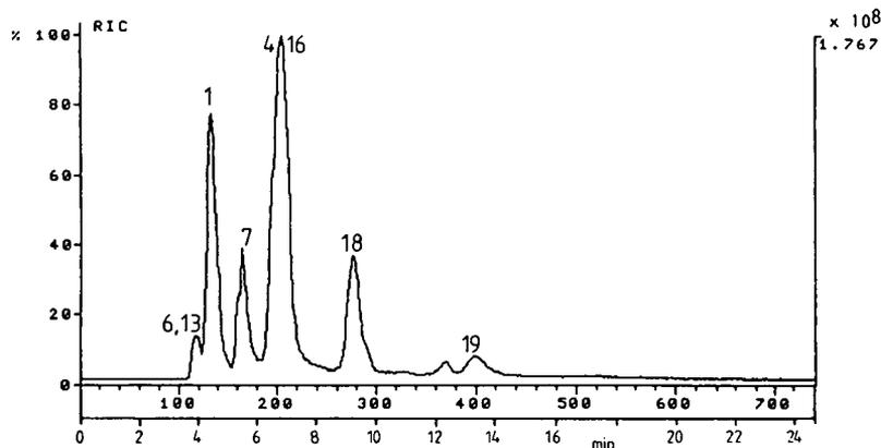
Fig. 6. Total ion current chromatogram of an LC–particle-beam-MS analysis of sample B. For conditions, see Experimental.
