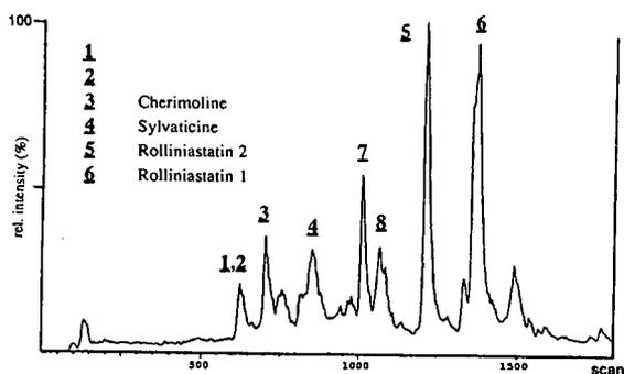
Fig. 5. LC-TSP-MS analysis of acetogenins from *Annona purpurea*. Column, Nucleosil C<sub>18</sub>, eluent CH<sub>3</sub>CN–H<sub>2</sub>O gradient from 60:40 to 85:15, flow-rate, 1 ml/min; detection UV at 208 nm, TSP vaporizer, 90°C; source, 250°C; filament off; buffer, 0.5 M CH<sub>3</sub>COONH<sub>4</sub> at 0.2 ml/min.
