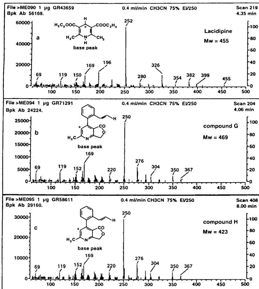
Fig. 4. PB-EI mass spectra of: (a) lacidipine; (b) compound G; (c) compound H.
