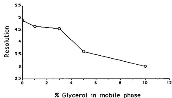
Fig. 5. Effect of concentration of glycerol in the mobile phase on the resolution ( $R_s$ ).  $\circ$  = Met-enkephalin;  $\square$  = leu-enkephalin.
