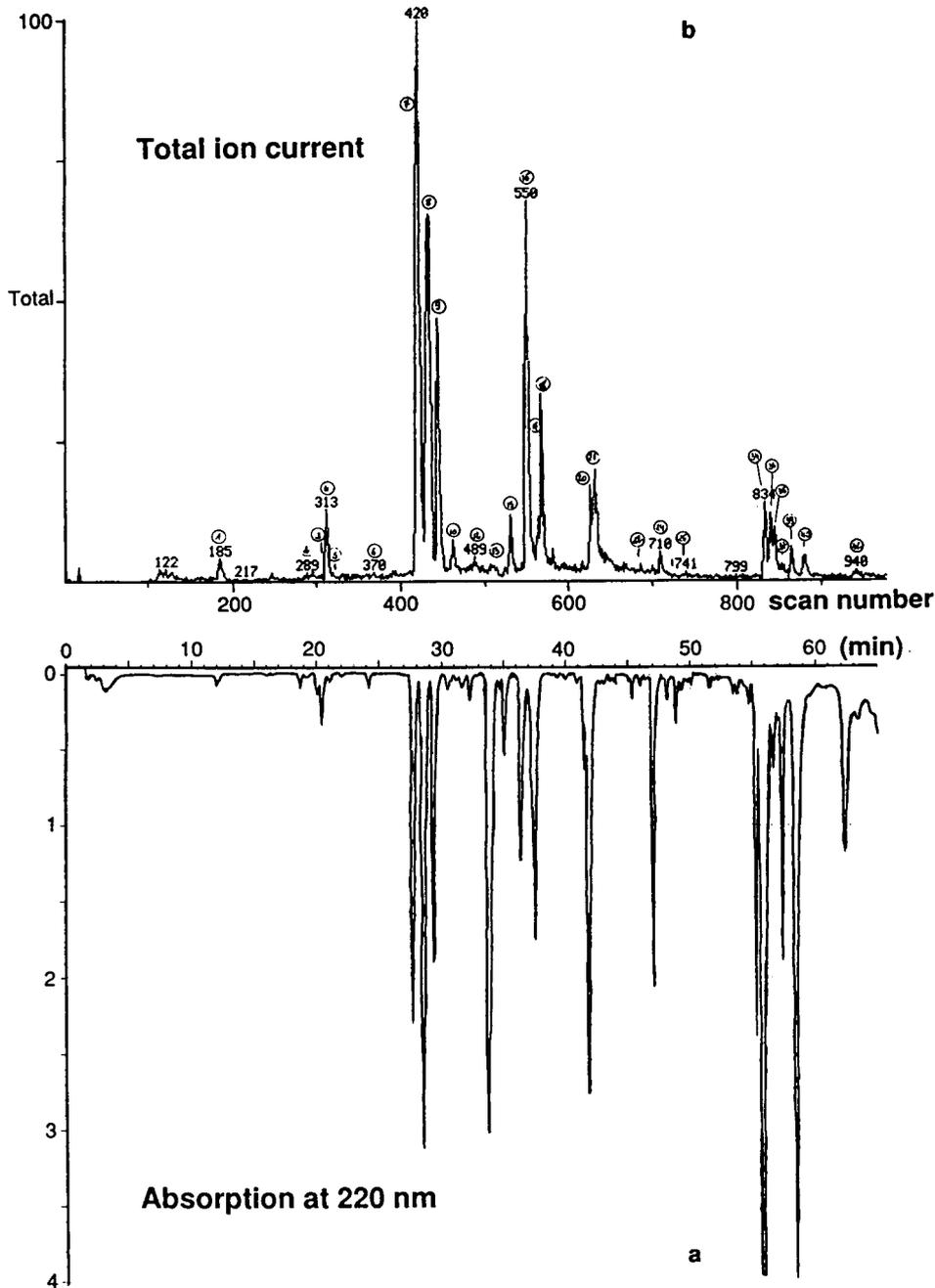
Fig. 2. Peptide map of rhIFN- $\gamma$ . (a) Detection by UV absorbance at 220 nm; (b) detection by total ion current.
