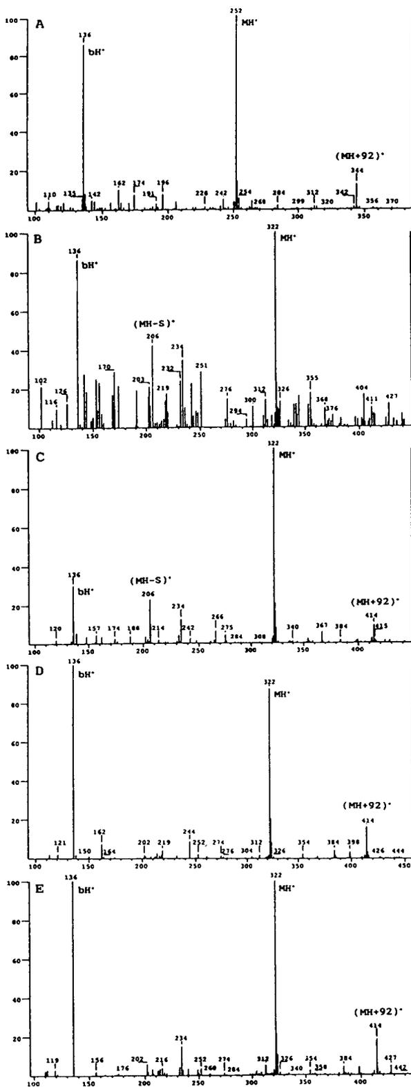
structure. All the spectra contain an abundant protonated molecule and also glycerol adduct ion. The spectrum of peak A exhibits an abundant protonated molecule of dAdo ( $m/z$  252) and an ion at  $m/z$  136 ( $bH^+$ ) formed by the cleavage of the glycosidic bond with hydrogen transfer. The spectra of the other peaks (B-E) exhibit abundant protonated molecules of BM adducts of dAdo ( $m/z$  322), indicating the formation of isomeric adducts.
