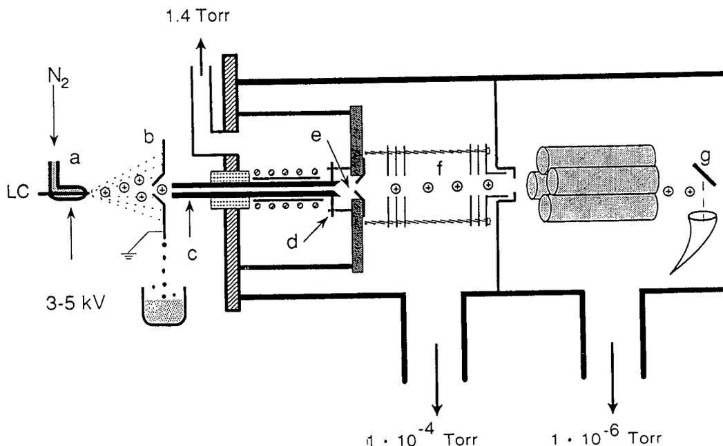
Fig. 1. General schematic of the ion spray LC–MS system incorporated on an HP 5985B mass spectrometer. a = Ion spray; b = liquid shield; c = heated ion capillary; d = centering device; e = skimmer; f = Einzel lenses; g = high-energy dynode detector. 1 Torr = 133.322 Pa.
