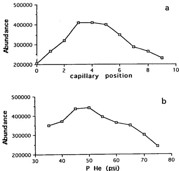
Fig. 1. Effect on peak abundance of  $\text{HRu}_3(\text{C}\equiv\text{C-tert-Bu})(\text{CO})_2$ , of: (a) position of the end of the capillary in the nebulizer (arbitrary setting units); (b) nebulizing gas helium pressure. Operating conditions: FIA; eluent, methanol; flow-rate, 0.4  $\text{cm}^3/\text{min}$ ; source temperature, 260°C.
