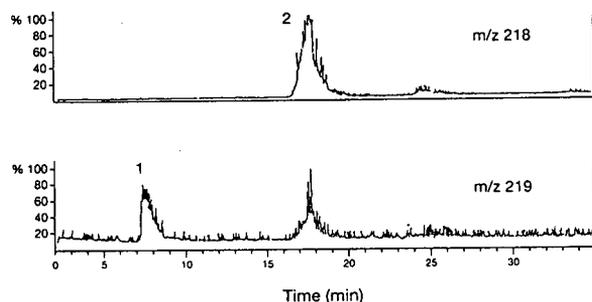
Fig. 4. Mass chromatograms of a Val-NH<sub>2</sub> sample from an enzymatic hydrolysis experiment. Peaks: 1 = Val; 2 = Val-NH<sub>2</sub>. Mobile phase, 0.1 M triethylammonium formate and 8 mM NDFA. For other conditions, see Experimental.
