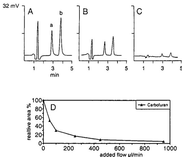
Fig. 6. LC–UV response of monuron (a) and carbofuran (b) with post-column addition on a  $100 \times 1$  mm I.D. column (see Experimental for conditions). (A) No post-column addition; (B) 50  $\mu$ l/min post-column addition; (C) 450  $\mu$ l/min post-column addition; (D) summary of LC–UV response for carbofuran with various post-column additions of column eluent.
