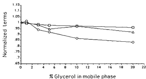
Fig. 2. Influence of glycerol on the normalized efficiency, capacity factor and selectivity terms in partition chromatography (system A). ○ =  $\sqrt{N_x}/\sqrt{N_0}$ ; □ =  $f(k')_x/f(k')_0$ ; △ =  $f(\alpha)_x/f(\alpha)_0$ .
