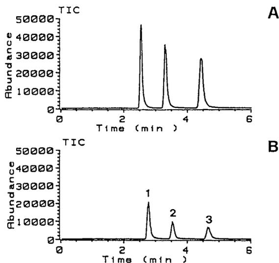
Fig. 5. High-flow ion spray *versus* conventional ion spray of alkyl benzoate esters on a  $100 \times 4.6$  mm column SIM of  $m/z = 151, 165, 179$  ( $\text{MH}^+$ ), dwell time = 300 ms. (A) High-flow ion spray without post-column split and liquid shield; (B) conventional ion spray with post-column split and no liquid shield.
